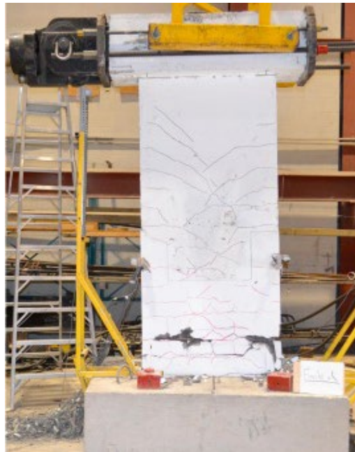
Figure 5. Cracking pattern of R-SWN-Z at end of testing [3].
