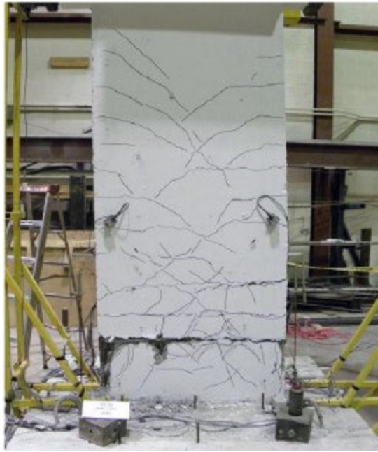
Figure 4. Cracking pattern of SWN-A after 72 mm (3.0% drift cycle)[1].
