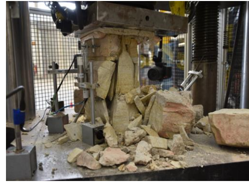
Figure 5: Stone prism compression test
