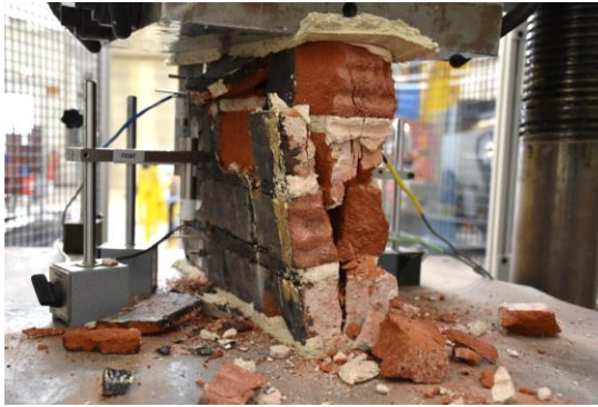
Figure 4: Brick prism compression test
