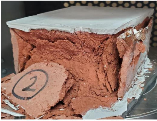
Figure 2: Brick unit compression test
