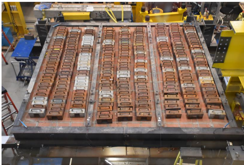
Figure 8: Hollow terracotta floor tile diaphragm reversed cyclic lateral load testing
