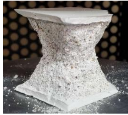
Figure 3: Mortar sample compression test
