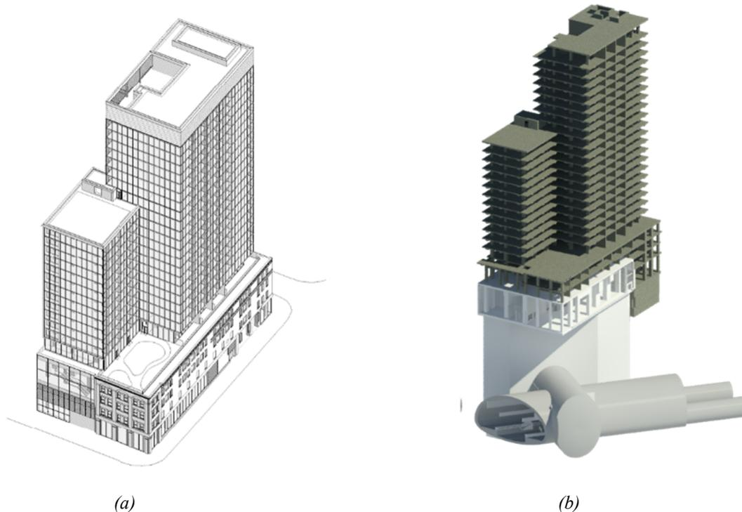
Figure 1. 3D view of 27 storey TOC overbuild and 3 storey transit station: (a) Architectural rendering, (b) Structural rendering with TOC structure (in gray) and station elements (in white).
