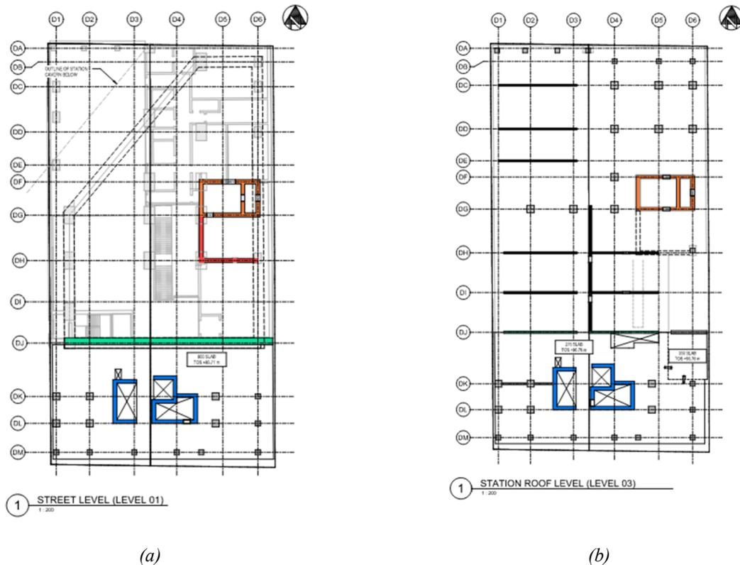
Figure 3. Structural wall layout: (a) Street Level, (b) Level 03 (Station Roof)
