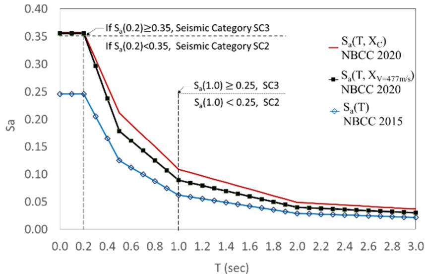
Figure 2. Design spectrum for TOC site based on NBCC 2015 and NBCC 2020
