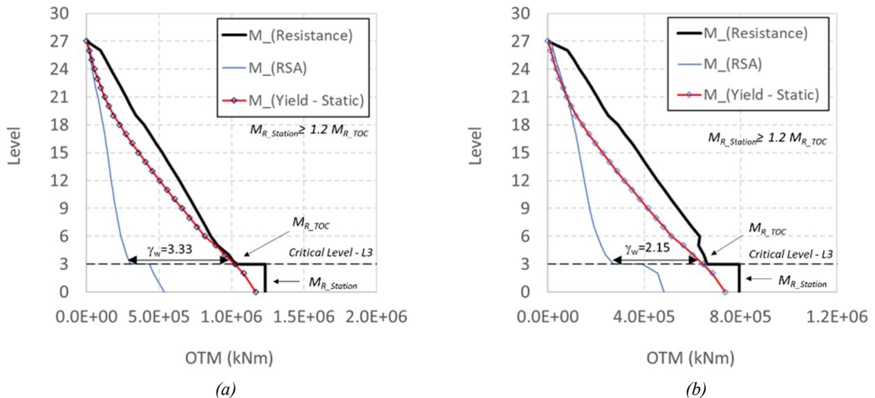
Figure 5. Moment resistance, moment demand and moment at yield plots: (a) X direction, (b) Y direction
