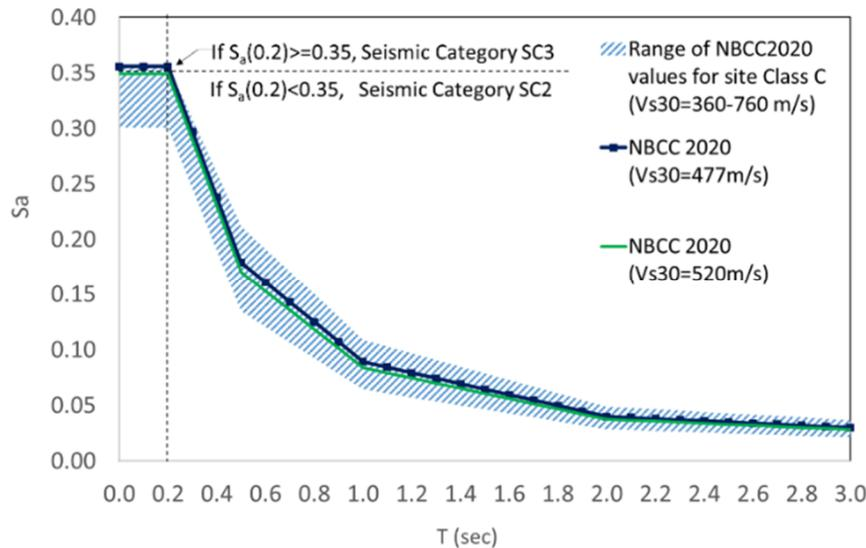
Figure 6. Variation of TOC design spectrum vs shear wave velocity,  $V_{S30}$
