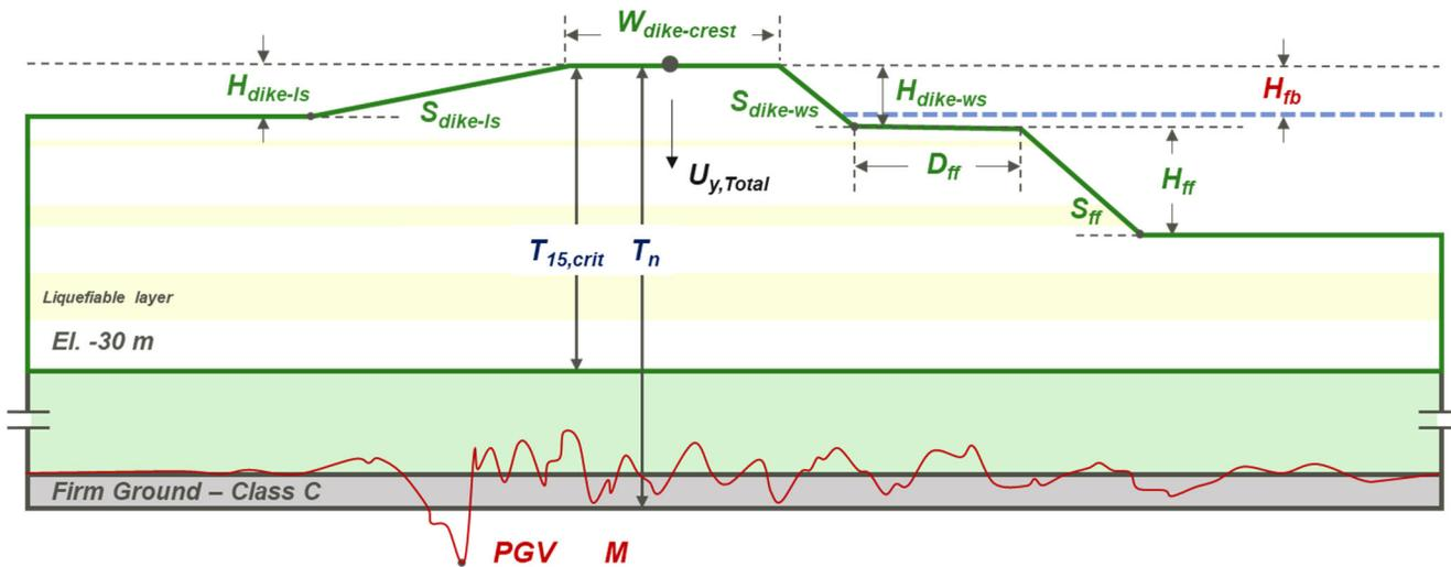
Figure 5. Schematic of response model input parameters.
