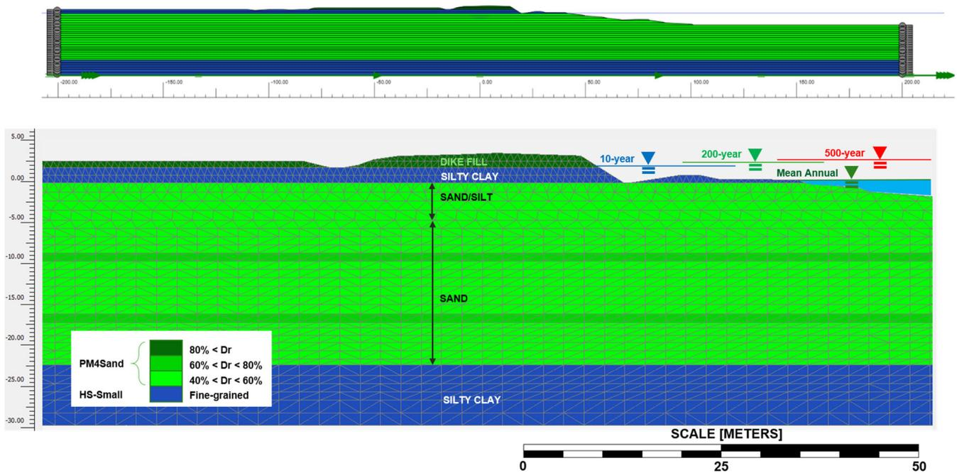
Figure 1. Example of typical PLAXIS cross section and distribution of constitutive models.
