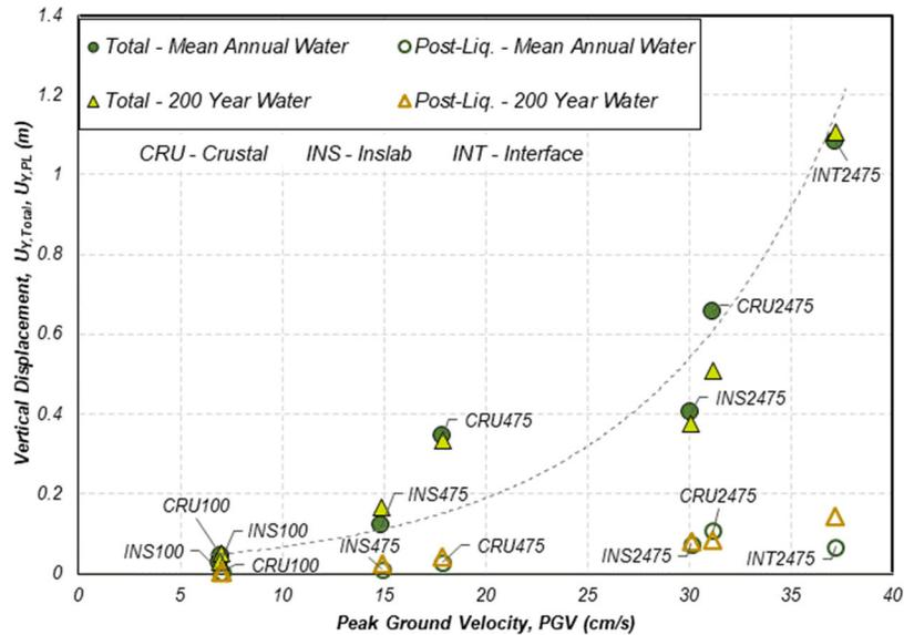
Figure 3. Summary of total and post-liquefaction settlement at one of the analyzed dike locations.
