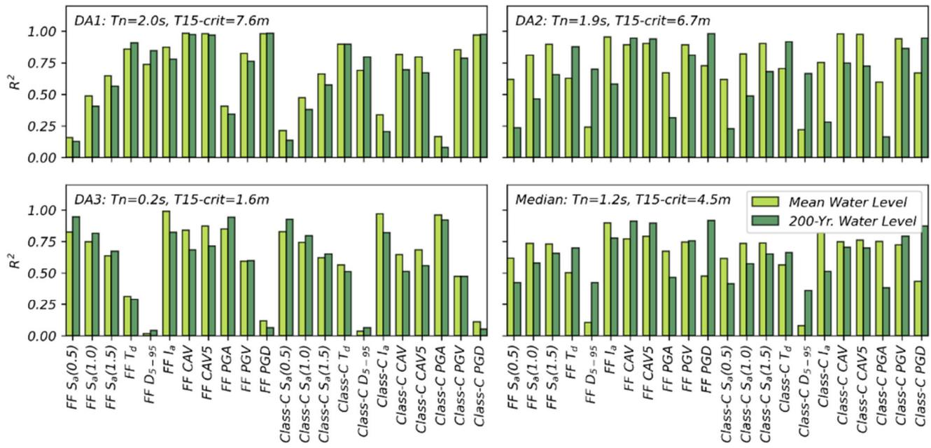
Figure 4. Efficiency of select IM metrics for mean and 200-year flood levels at three site locations (DA1, DA2 and DA3 in Table 1), and for the median of scores from individual sites as assessed by  $R^2$ . FF denotes free field, as in earthquake IMs correspond to level ground surface conditions. Class-C indicates that earthquake IMs correspond to the input base reference condition.
