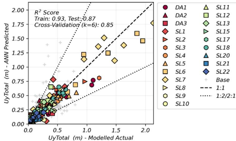
Figure 6. Comparison of predicted vs. actual total dike crest settlements using the ANN model. Grey symbols represent additional dike geometries that evaluated the effects of individual input variables on the response.
