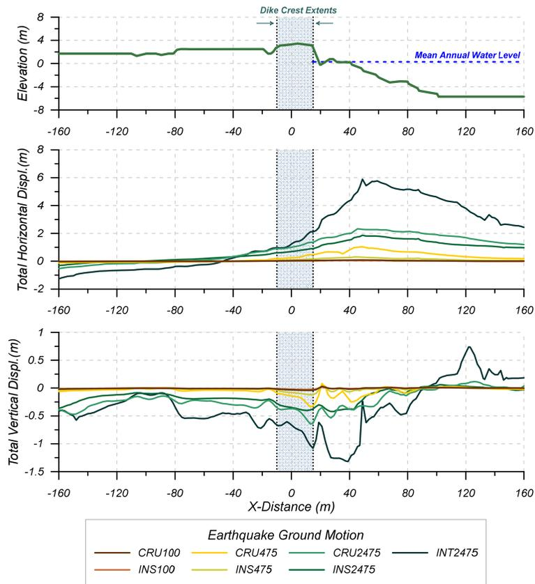
Figure 2. Total horizontal and vertical displacement with model distance for different earthquake ground motions at one of the analyzed dike locations, for mean annual water level.
