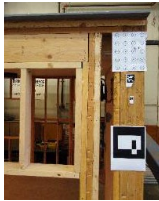
Figure 3 target placement on the specimen
