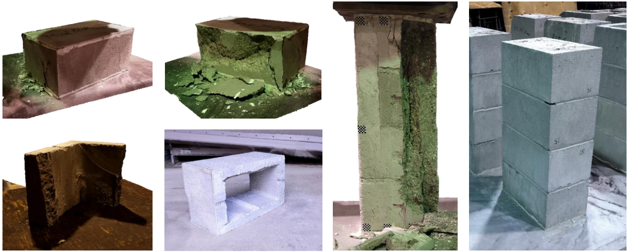
Figure 1. Samples of 3D reconstructed models of masonry blocks and prism before and after compression test under indoor or outdoor lighting conditions.
