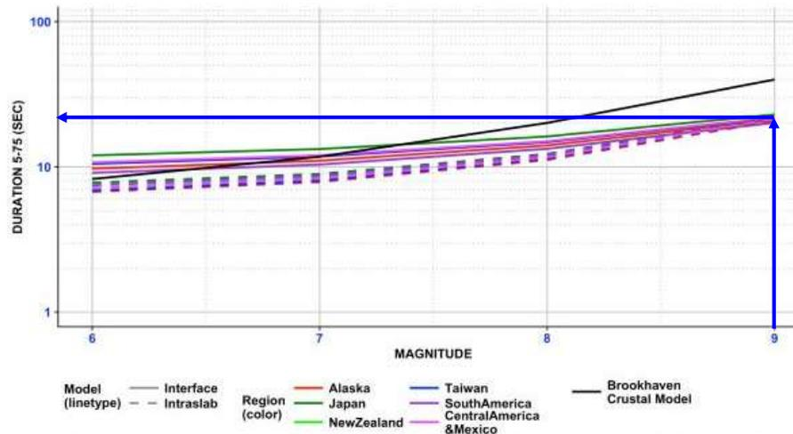
Duration model versus earthquake magnitude at  $R_{jb} = 100$  km. Solid lines are interface source-type, dashed lines are intraslab source-type, black line is Brookhaven (crustal model).
