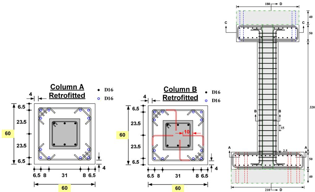
Figure 3. Column section and detailing of test specimens.
