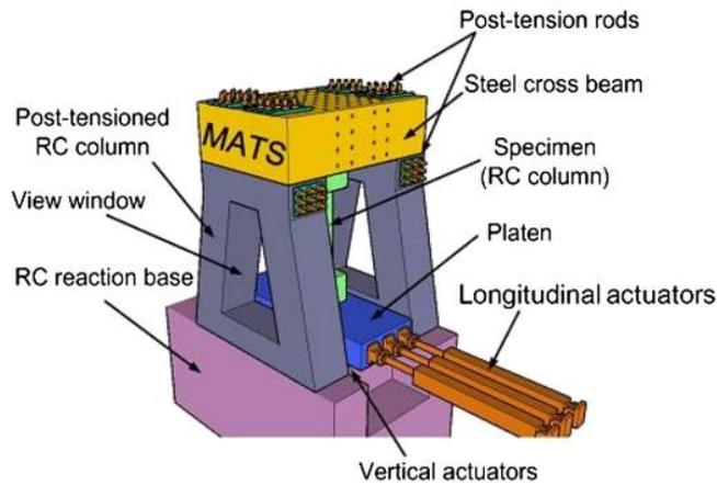
Figure 4. Test setup of RC column at the multi-axial testing system (MATS)[4] in NCREE.
