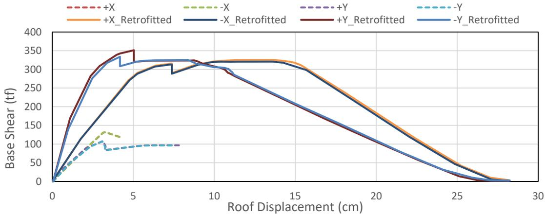
Figure 12. The base shear–roof displacement curves of the school building before and after retrofitting.
