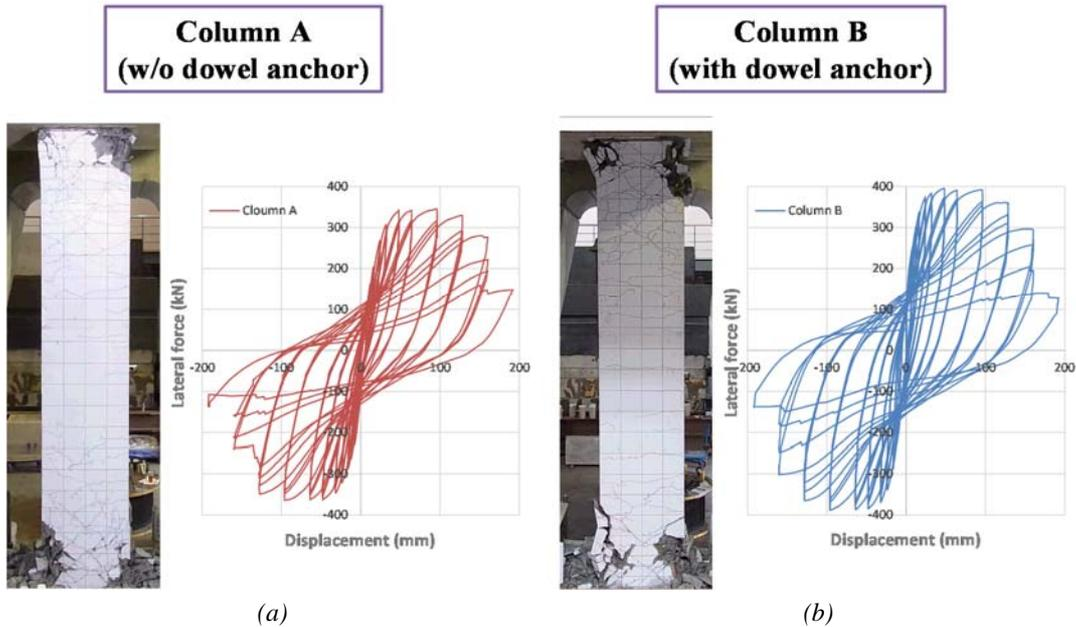
Figure 6. Test results of jacketed columns: (a) without dowel anchor, (b) with dowel anchor.
