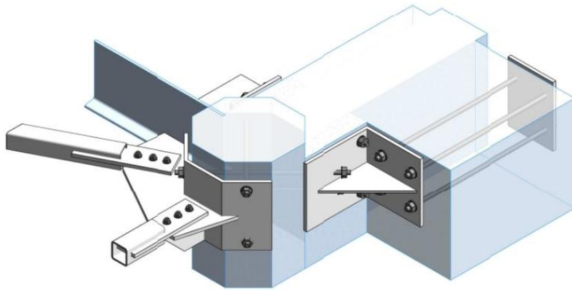
Figure 9. Horizontal steel braced frames connected to a hexagonal RC column.
