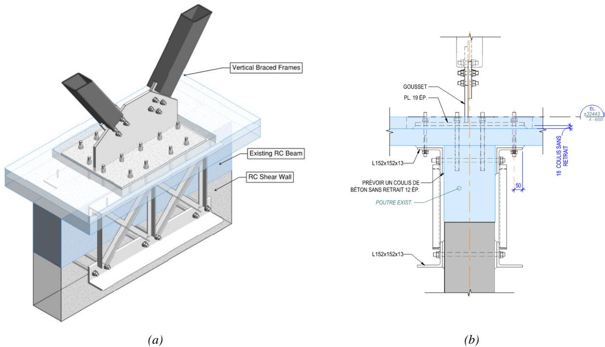
Figure 10. Steel truss used as a force transferring mechanism: (a) 3D view, (b) Section view
