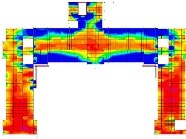
*Figure 4. Example of a numerical analysis of building ensemble SABC diaphragm axial stresses*
