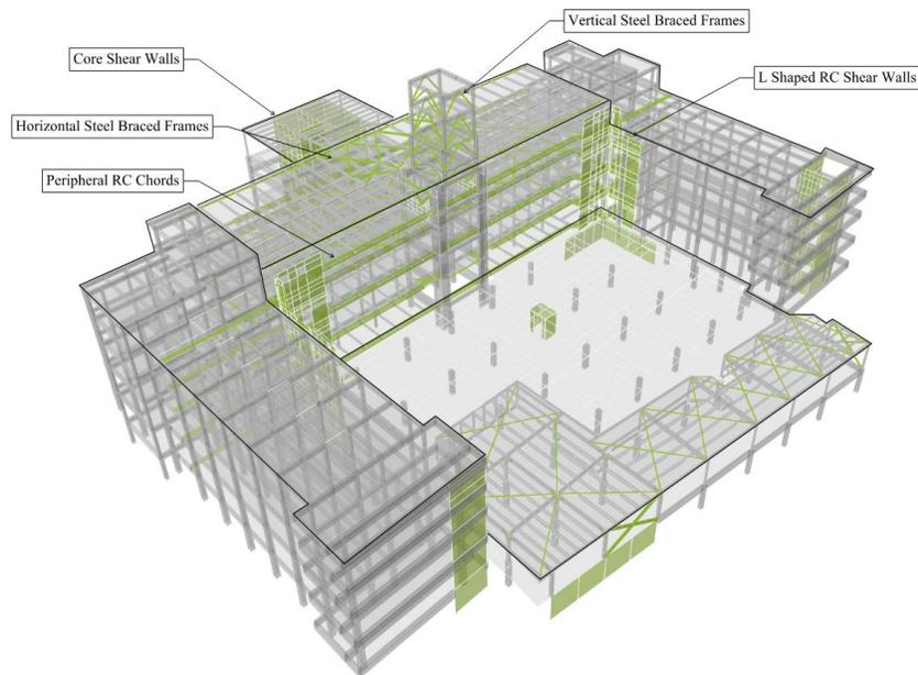
Figure 5. Numerical Etabs model featuring the implemented retrofit solution for building ensemble SABC
