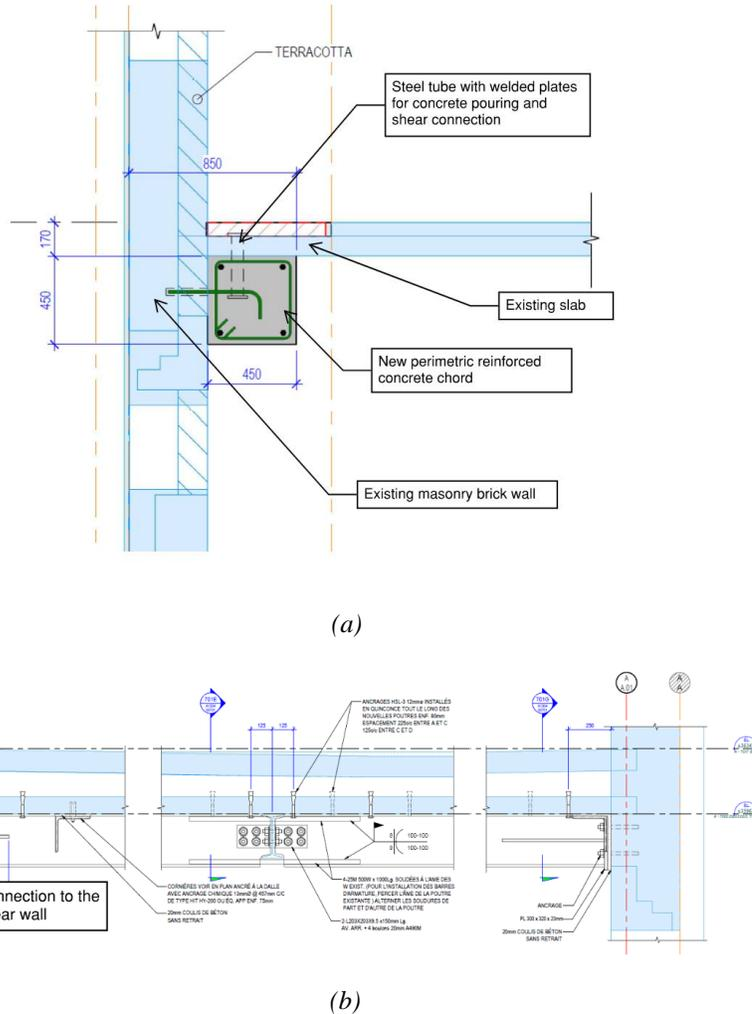
Figure 7. Diaphragms retrofit solutions (a) New peripheral reinforced concrete chords; (b) New added collectors beams
