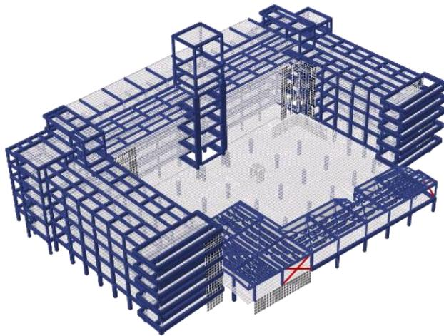
Figure 3. Initial model used for the seismic assessment; masonry walls are not shown for simplicity purposes
