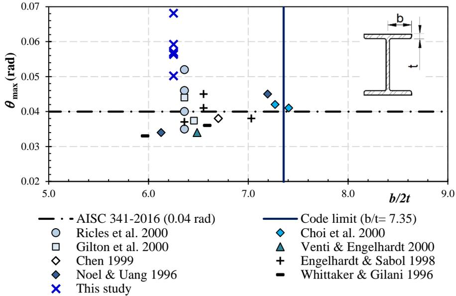
Fig. 4. Plastic rotation as a function of the flange beam slenderness
