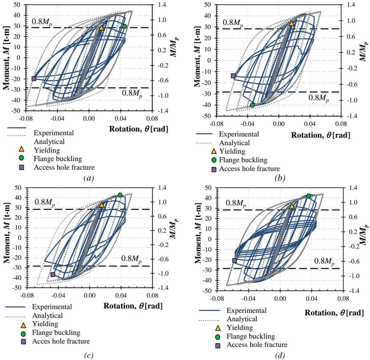
Fig. 6. Hysteretic curves (a) Specimen CTA-1; (b) Specimen CTA-2; (c) Specimen CPA-1; (d) Specimen CPA-2
