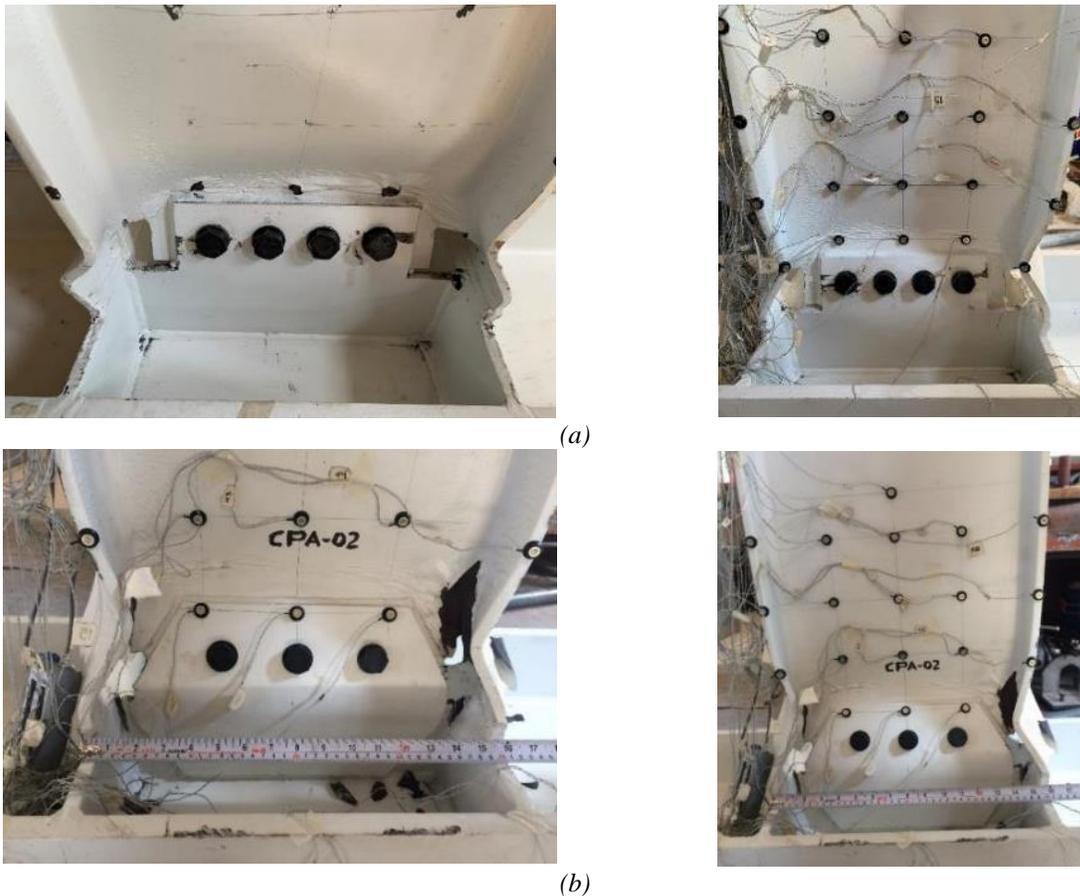
Fig. 3. Damage concentration, (a) Typical state of Specimen CTA; (b) Typical state of Specimen CPA
