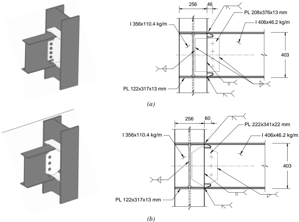
Fig. 1. Studied configurations: (a) Specimen CTA, (b) Specimen CPA
