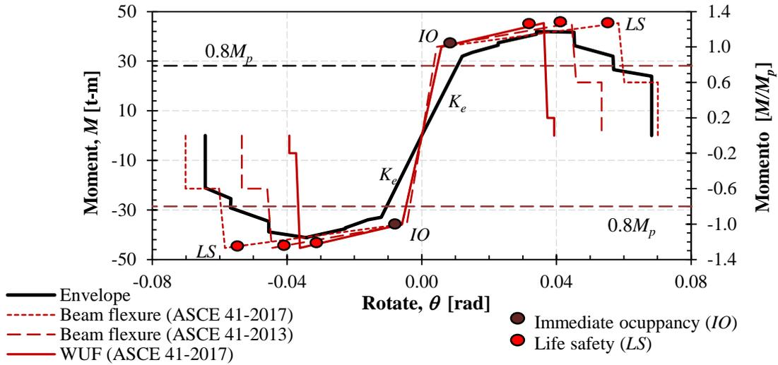
Fig. 10. Idealized force-displacement curves and enveloping curve
