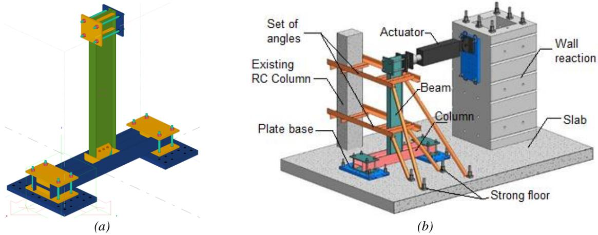
Fig. 2. Configuration, (a) Specimen, (b) Test configuration
