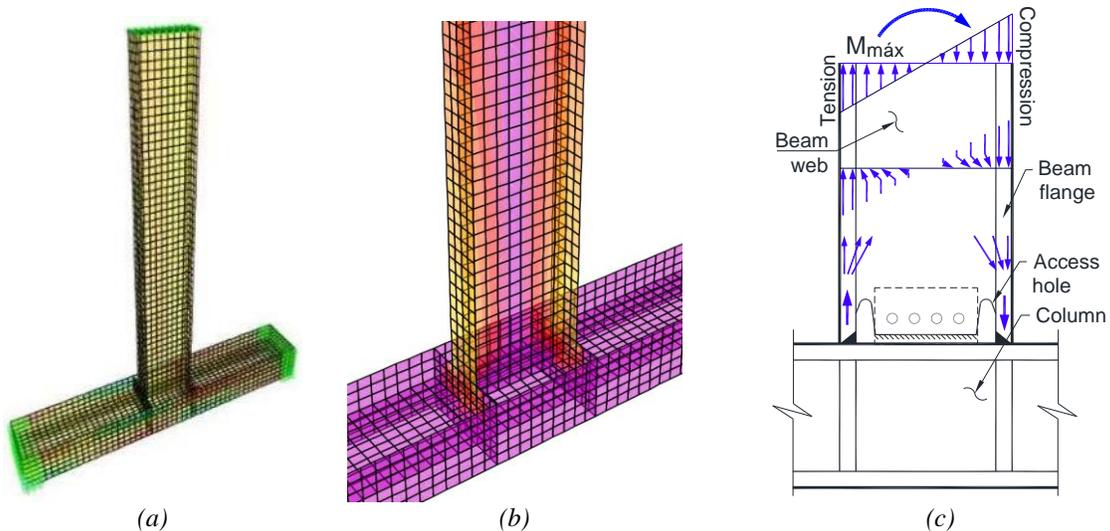
Fig. 5. Analytical model (a) Studied model, (b) Stress distribution, (c) Concentration on flange beam
