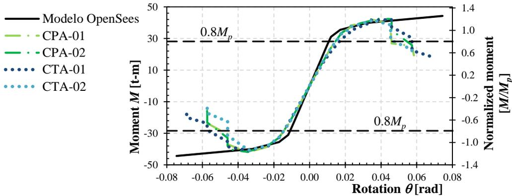
Fig. 8. Capacity curve and enveloped experimental response
