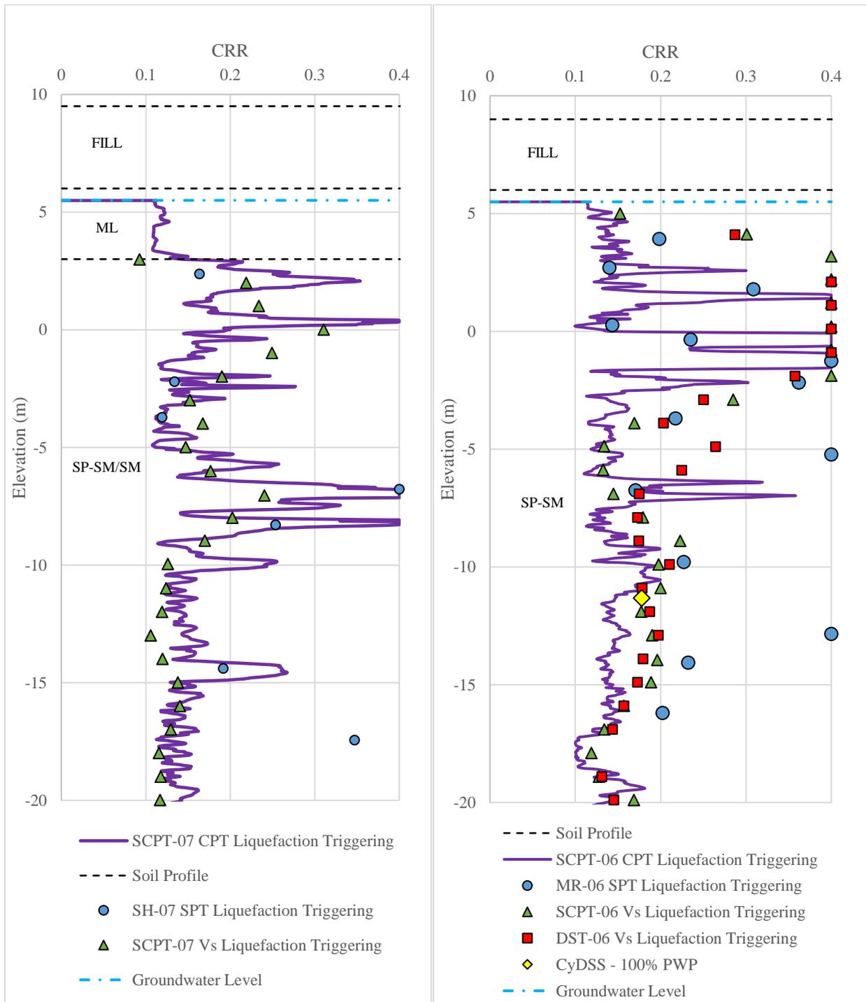
Figure 2: Comparison of Liquefaction Triggering Methods in Sonic (left) and Mud Rotary (right) Boreholes
