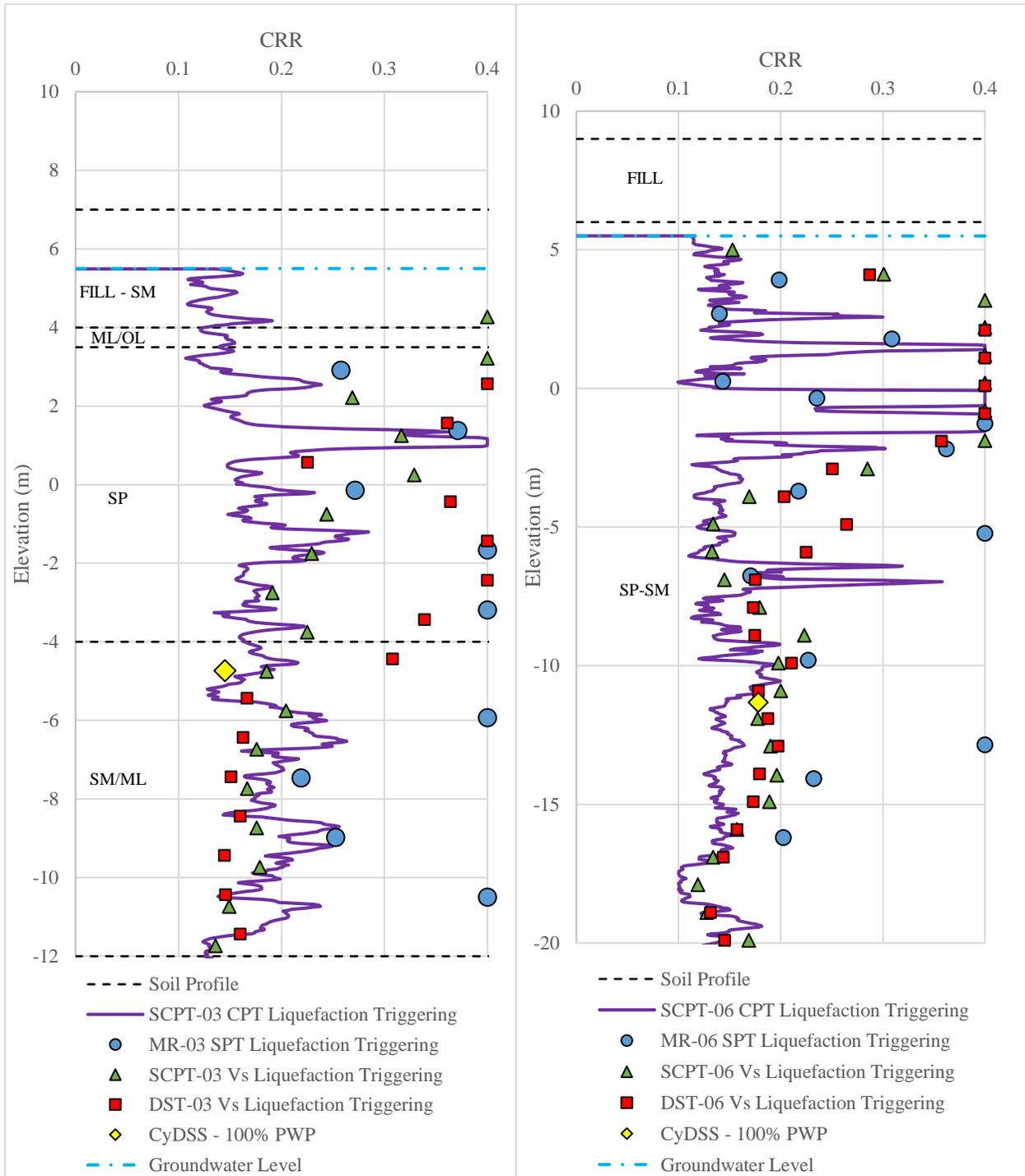
Figure 1: Comparison of Liquefaction Triggering Methods in Two Paired Mud Rotary Boreholes
