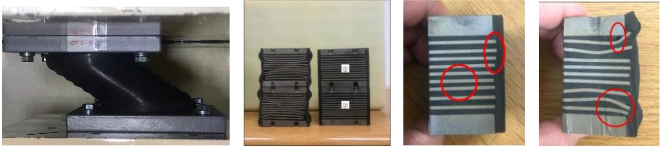
Figure 4. Shapes of LRB test and cross sections before and after the static tests
