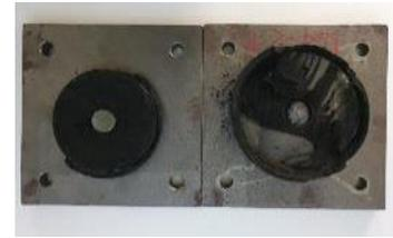
Figure 11. Shapes of isolation system break by BDBE (PGA:0.6g).
