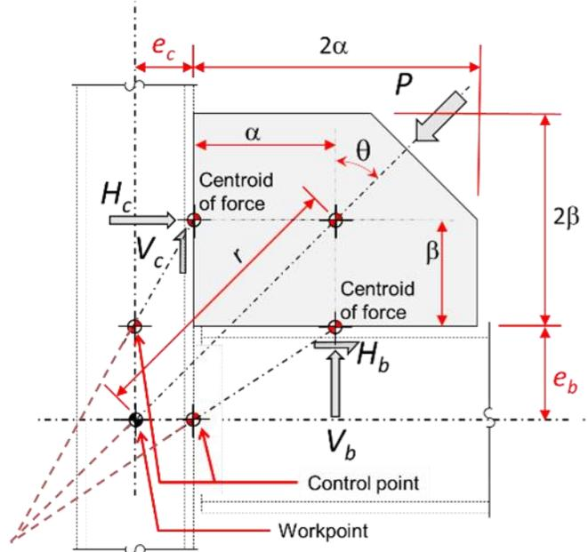
Figure 1. Uniform Force Method dimensions
