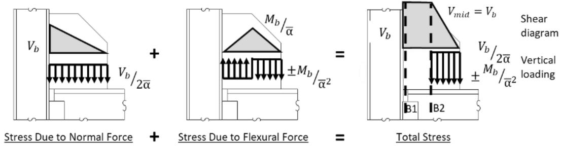
Figure 3. Stress distribution in beam due to normal force and moment.
