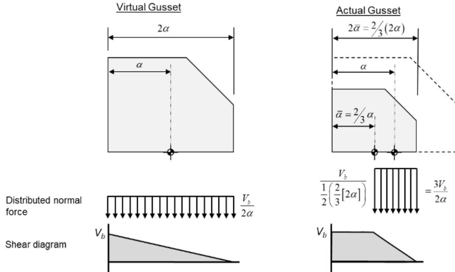
Figure 4. Distribution of normal force and corresponding shear diagrams for virtual and actual gussets.
