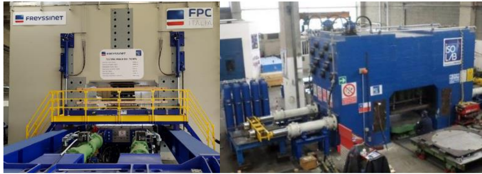
Figure 4. Test benches at ISOLAB: a) 70 MN; b) 50 MN
