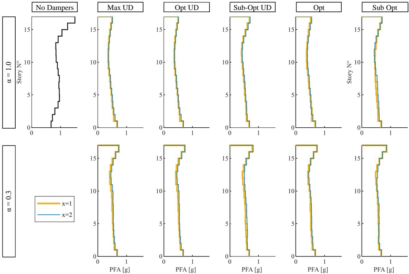
Figure 11. PFAs with optimal VD distributions.
