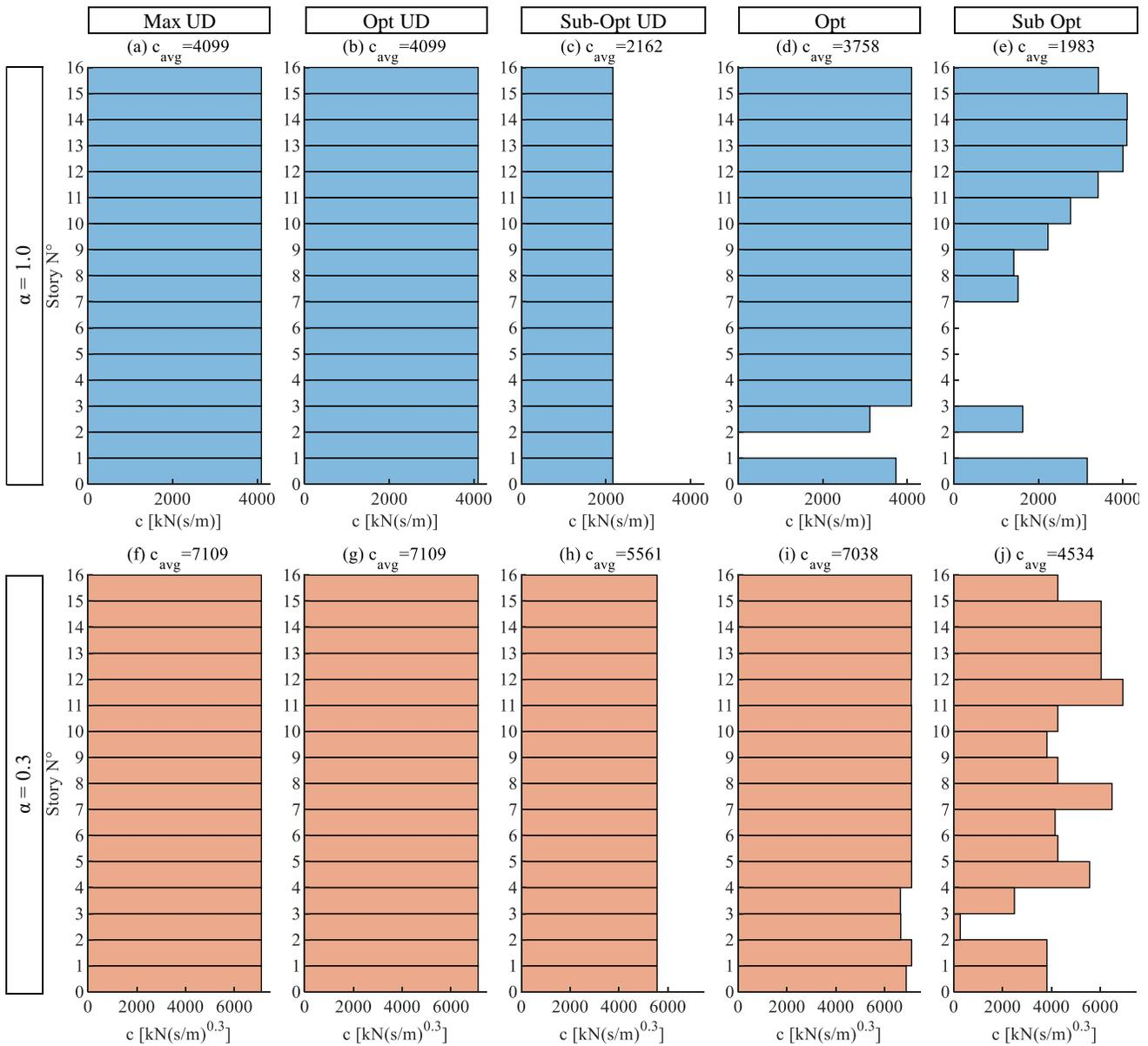
Figure 7. Optimal height-wise distributions of dampers spanning 1 story ( $x=1$ ).
