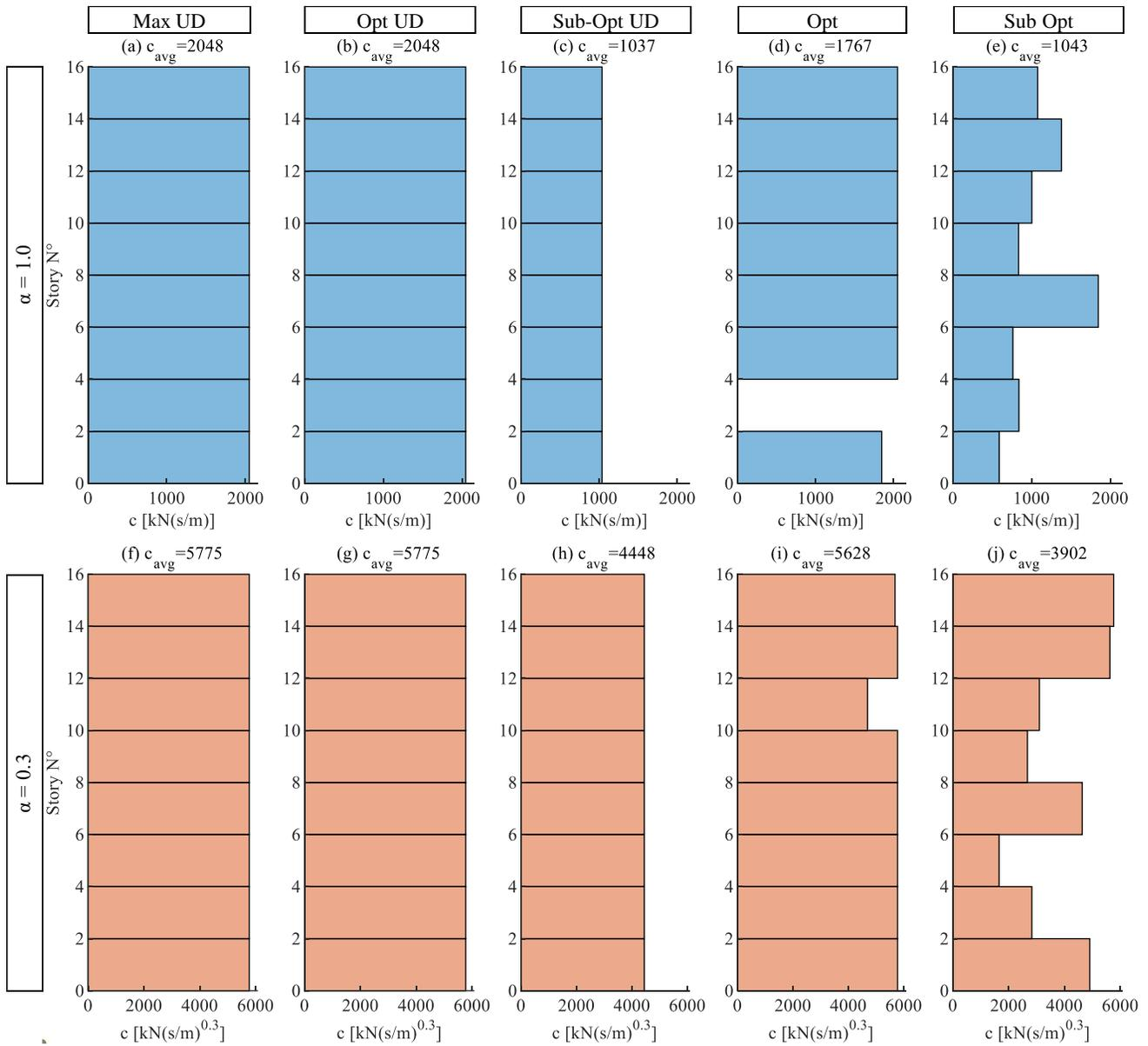
Figure 8. Optimal height-wise distribution of dampers spanning 2 stories ( $x=2$ ).
