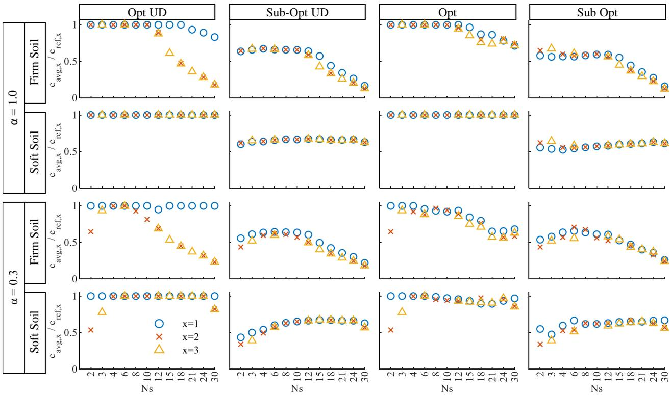
Figure 5. Optimal damping constants (average over all stories).
