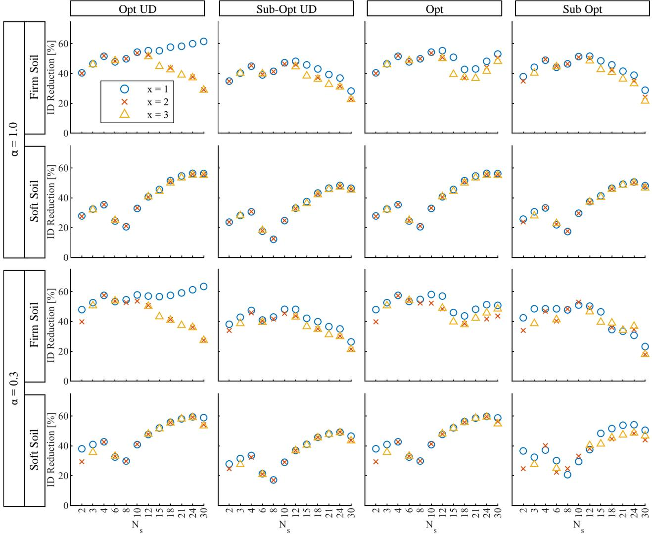
Figure 6. Inter story drift reductions achieved by the optimal solutions.
