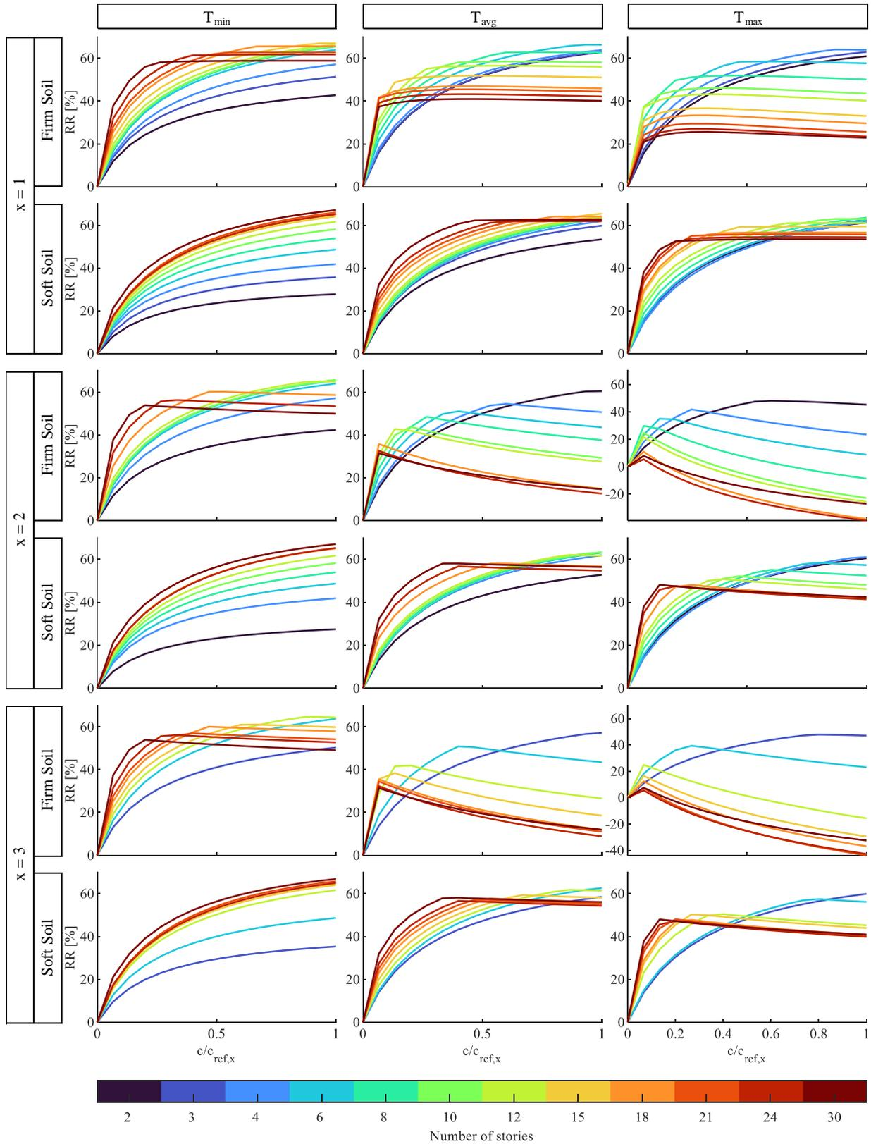
Figure 3. Evolution of RR vs.  $c$  with LVDs spanning  $x$  stories.
