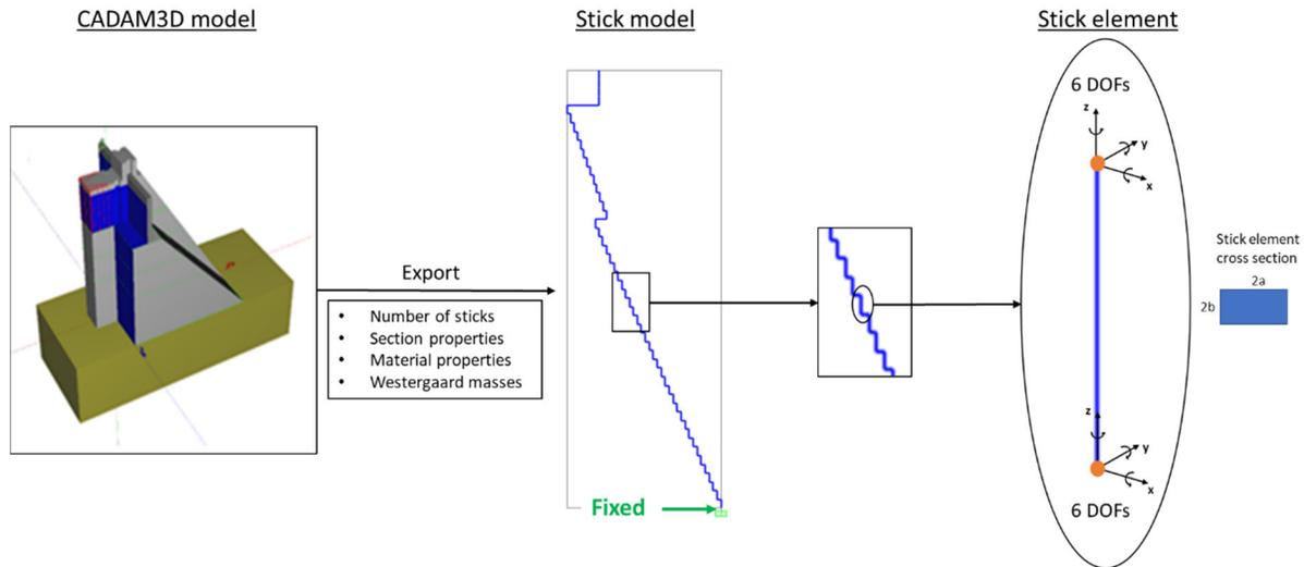
Figure 4. Creation of a stick model from a CADAM3D model.
