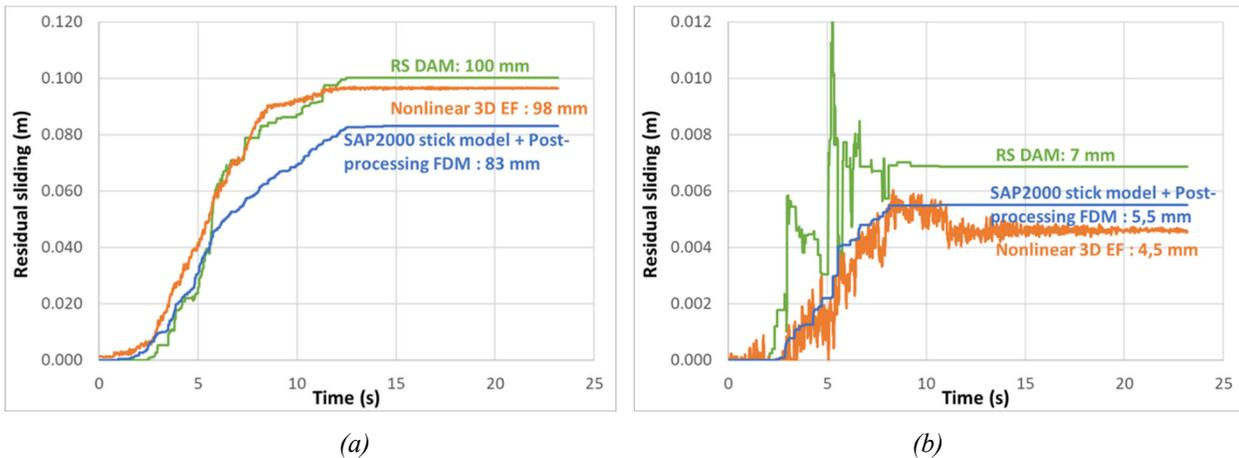
Figure 12. Comparison of the residual sliding at the joint  $H=90\text{m}$  : (a) upstream-downstream and (b) cross-valley
