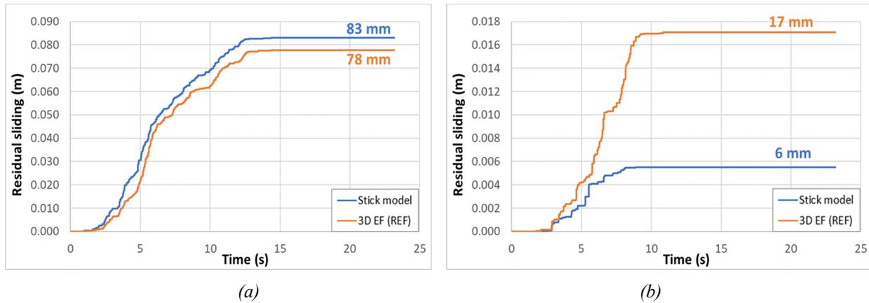
Figure 11. Comparison of the residual sliding at the joint  $H=90\text{m}$  computed with the FDM post-processor using linear forces from a linear transient analysis : (a) upstream-downstream and (b) cross-valley
