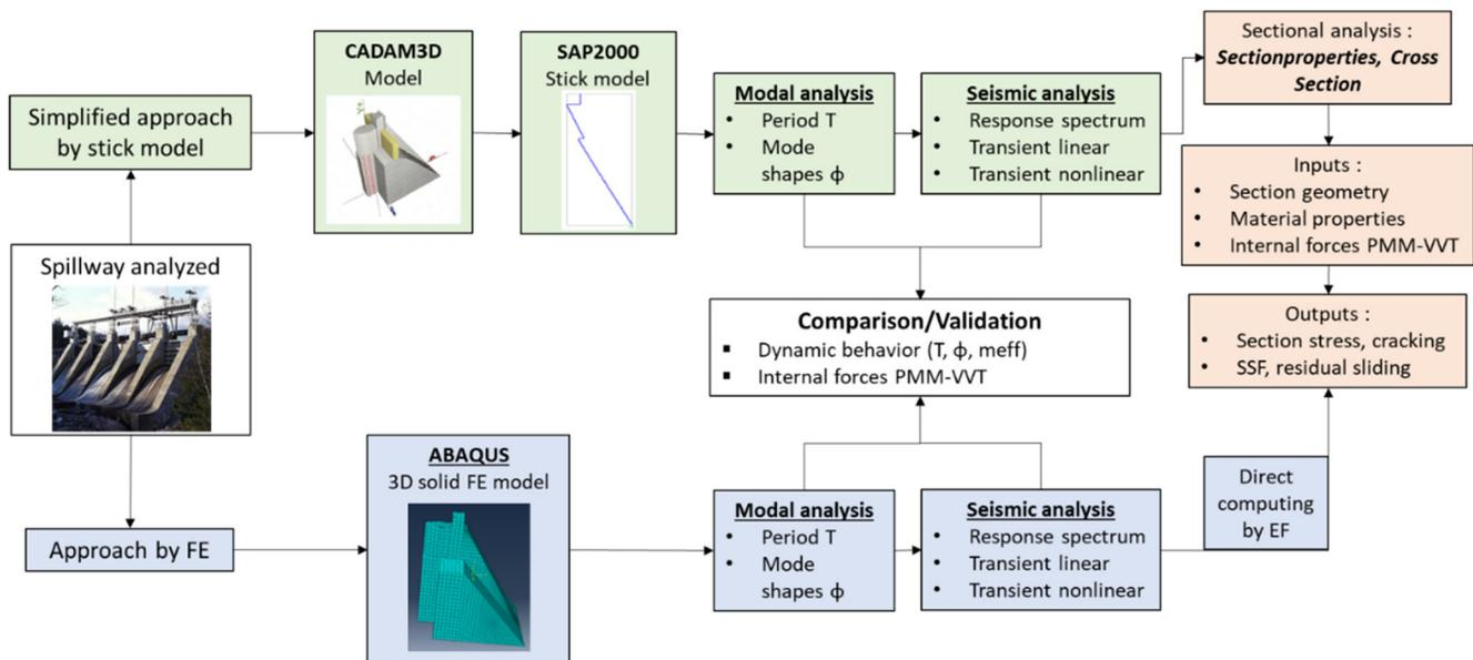
Figure 3. Flowchart of the stick model approach and its validation methodology.
