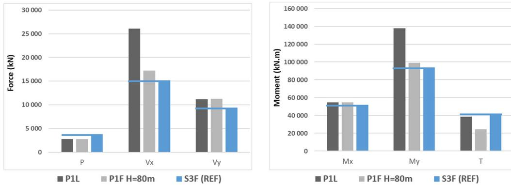
Figure 9. Comparison of internal forces and moments at the joint level  $H = 90\text{m}$  of the stick model P1L, the stick model fixed up to the level  $H=80\text{m}$  (P1F  $H=80\text{m}$ ), and the reference model S3F.
