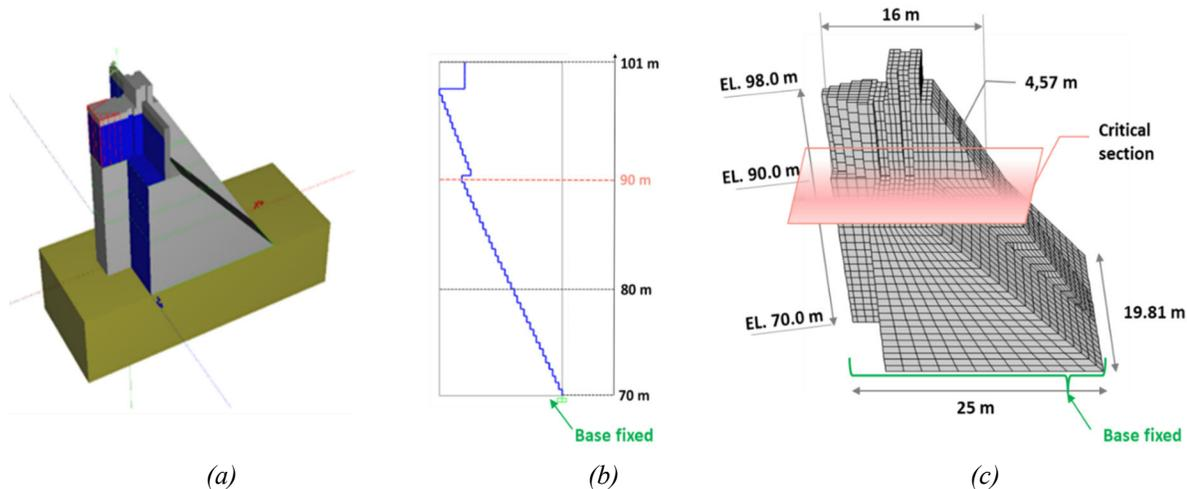
Figure 2. Different spillway pier models : (a) CADAM3D model, (b) Stick model (SAP2000), (c) 3D FE model (ABAQUS).
