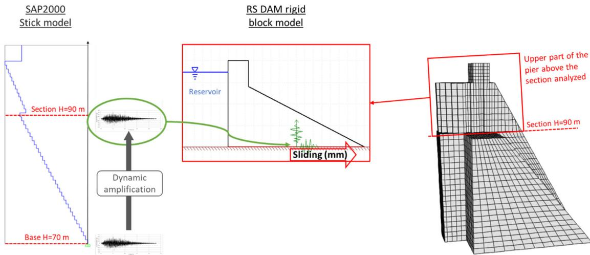
Figure 5. Crest block model and sources of excitation for the sliding stability analysis with RS-DAM.
