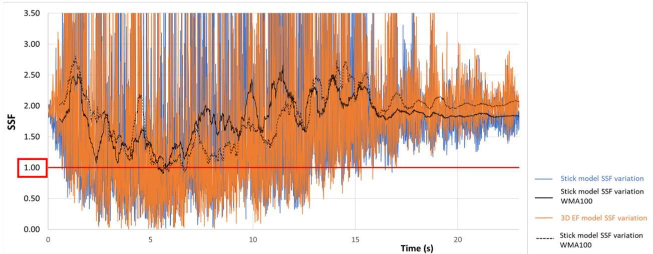
Figure 10. Comparison of the SSF variation curves of the stick model (in blue) with associated WMA curve (full black line) and the 3D FE model (in orange) with associated WMA curve (dotted black line).
