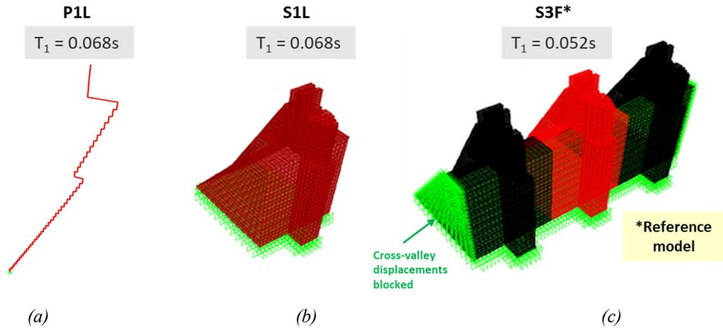
Figure 6. SAP2000 models analyzed and fundamental vibration periods: (a) stick model, (b) one pier solid model and (c) three piers solid model.
