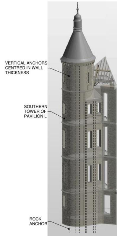
Figure 9. Rubble wall retrofit strategies considered: a) steel wall plate (typical plan detail); and b) schematic view of vertical anchors.
