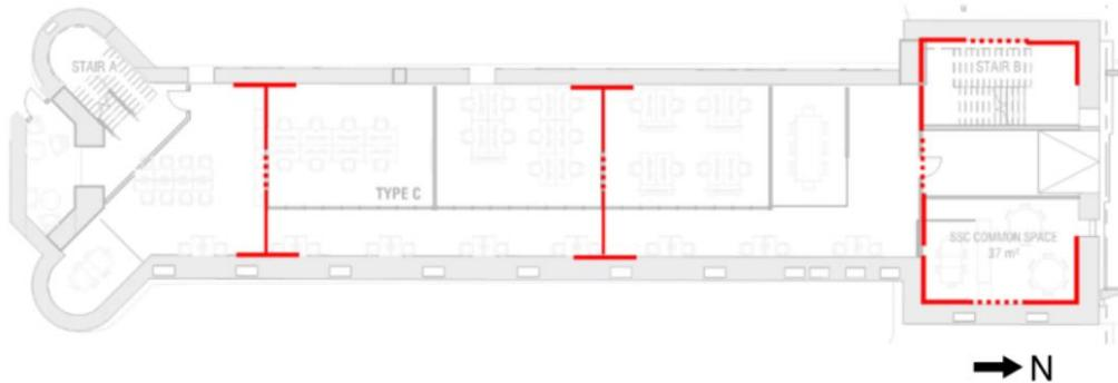
Figure 3. Preliminary design using concrete shear walls (in red).
