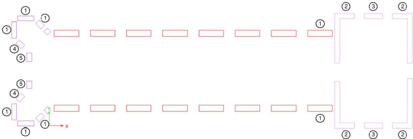
Figure 8. Map of the failing piers of the pavilion analyzed (note that the beams and floors are hidden for clarity).
