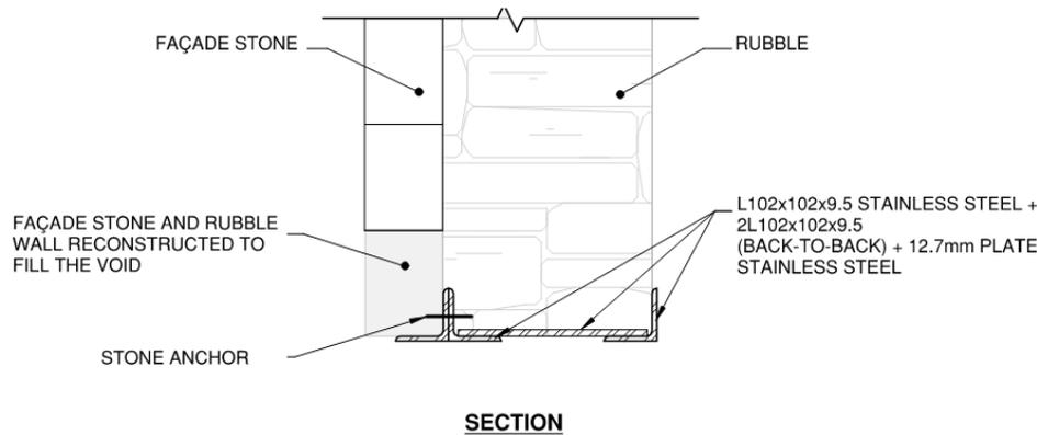
Figure 10. Spandrel retrofit strategy: post-installed steel lintels (typical detail).
