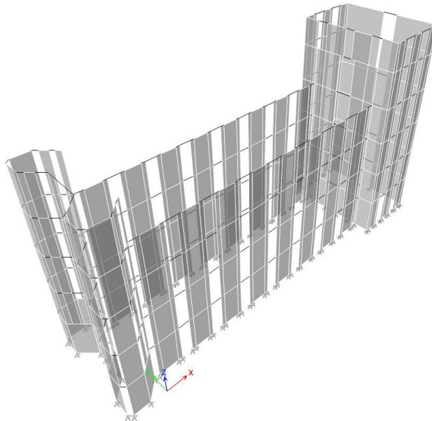
Figure 7. 3D view of the model proposed to perform the seismic analysis of the building.
