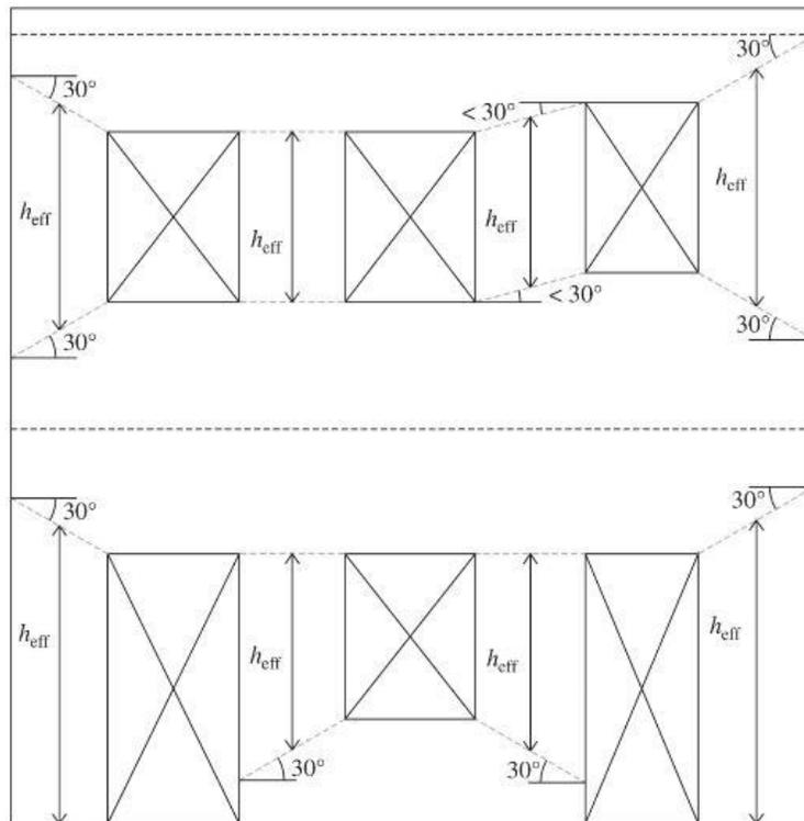
Figure 6. Figure C11-5 from ASCE 41 demonstrating the effective heights of wall piers. [4]
