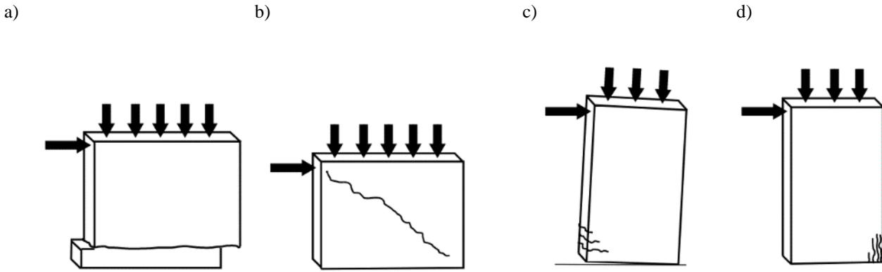
Figure 5. In-plane failure modes of a laterally loaded URM wall: a) bed-joint sliding; b) diagonal-tension; c) rocking; and d) toe-crushing.
