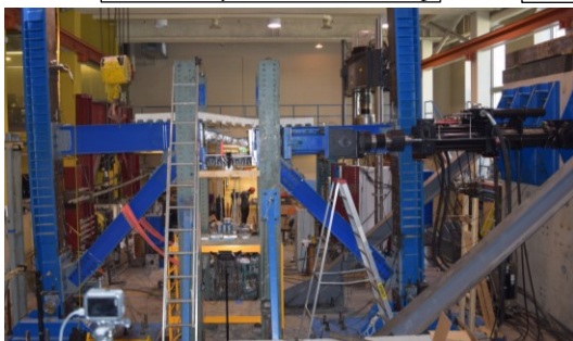
Frame Deformed Shape at 0.19 rads
