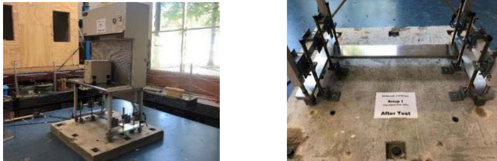
Figure 2. Test setup and EQRT 202 System installed on the equipment prior to testing.
