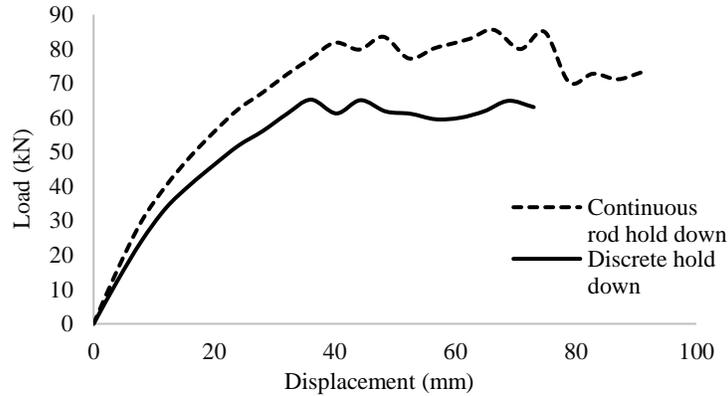
Figure 7. Comparison between push over curves in wood frame wall with different hold-down systems in SAP2000
