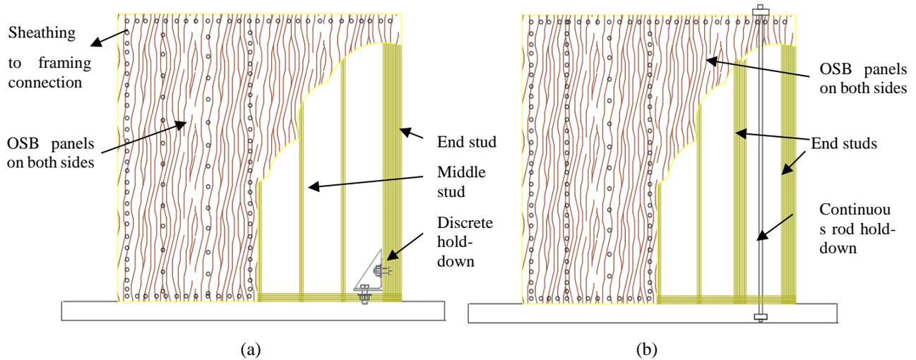
Figure 1. Configuration of (a) a wood frame shear walls with discrete hold-down, (b) a wood frame wall with continuous rods (reproduced with permission from [1], [2])
