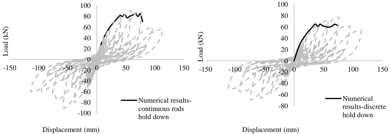
Figure 6. Comparison between the pushover curves of numerical wood frame shear walls with different hold-down systems in SAP2000 and cyclic curves of different hold-down systems from experiment [1], [4]
