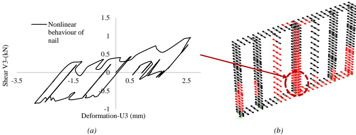
Figure 14. a) Nonlinear behaviour of one nail at the bottom of central stud, b) Location of max shear forces ( $0.85 < V < 1.37$  kN) in the first story shear wall under Loma Prieta Earthquake record in the model with continuous rods hold-down
