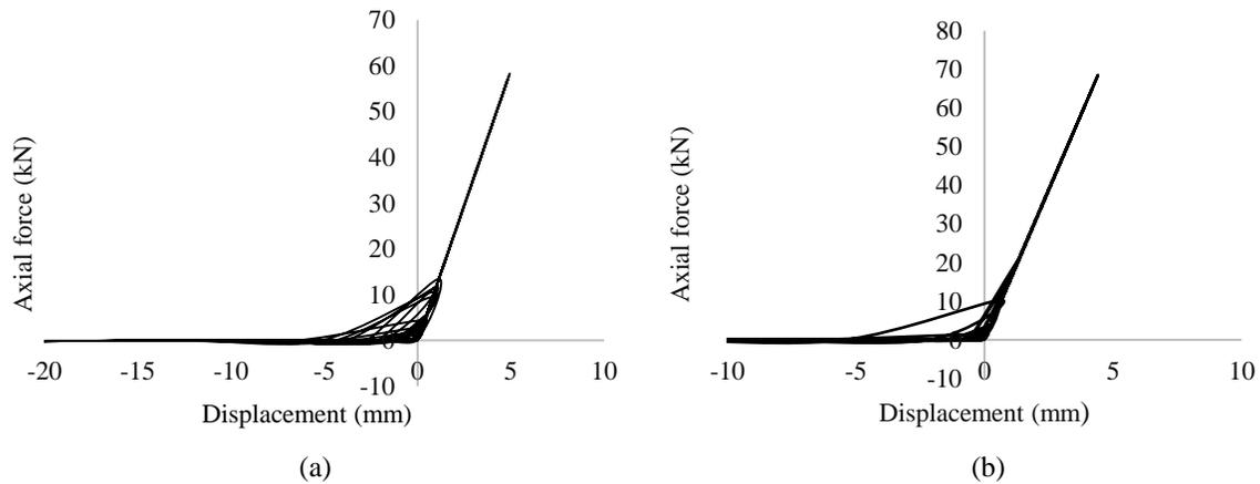
Figure 12. Behaviour of hold-down in walls with: (a) discrete and (b) continuous rods
