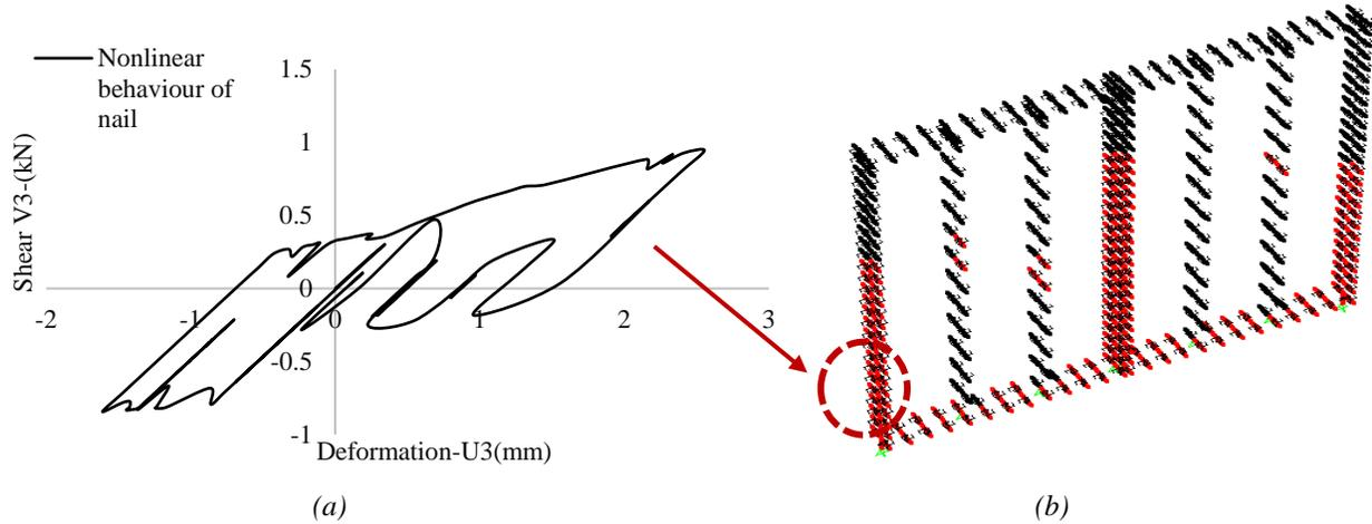
Figure 13. a) Nonlinear behaviour of one nail at the bottom of end stud, b) Location of max shear forces ( $0.85 < V < 1.19$  kN) in the first story shear wall under Loma Prieta Earthquake record in the model with discrete hold-down
