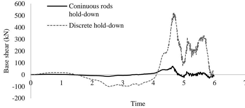
Figure 11. Base shear in the models with different hold-downs
