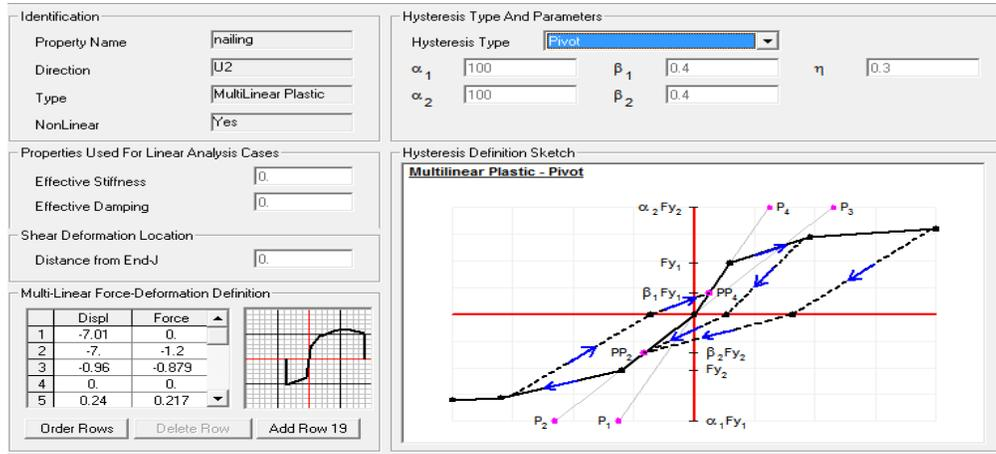
Figure 4. Nonlinear behaviour of the nail connections between sheathings and frames in SAP2000 obtained from Estrella et al. [1]
