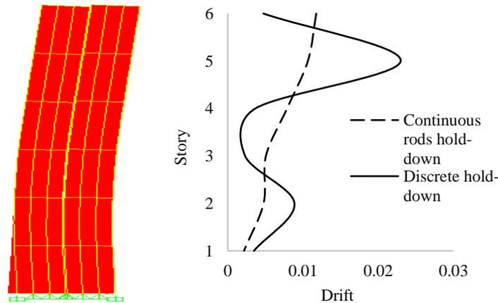
Figure 10. Inter-story drift in the models with different hold-downs
