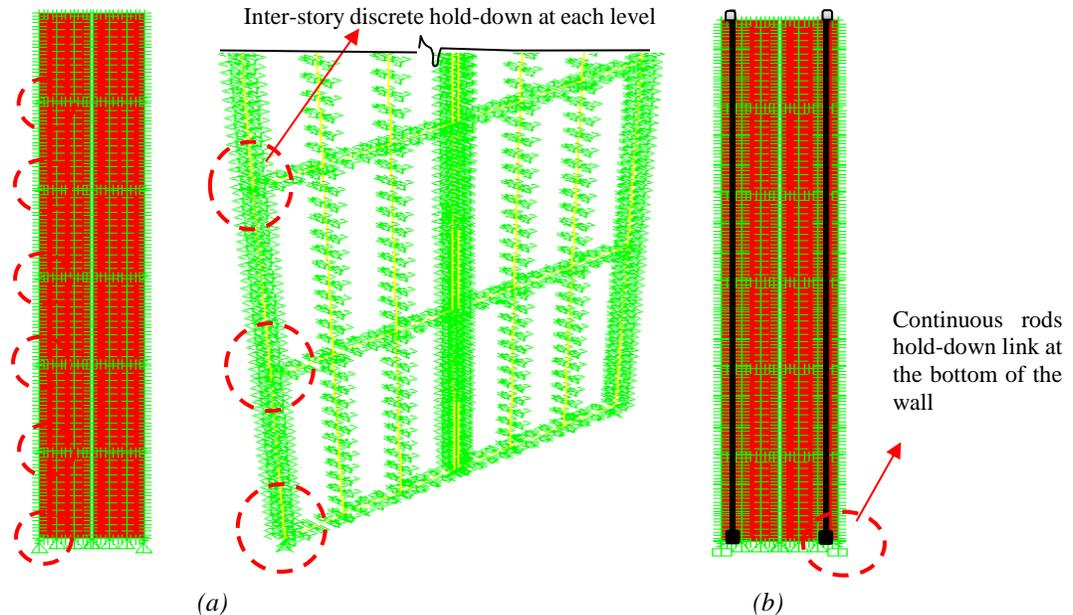
Figure 8. Numerical model for six-story wood frame shear wall with: (a) discrete hold-down, (b) continuous rods hold-down
