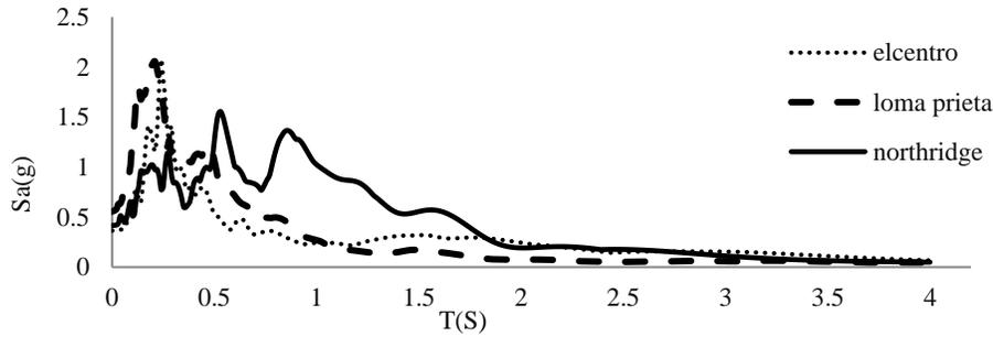
Figure 9. Horizontal acceleration spectra of the components with maximum PGA
