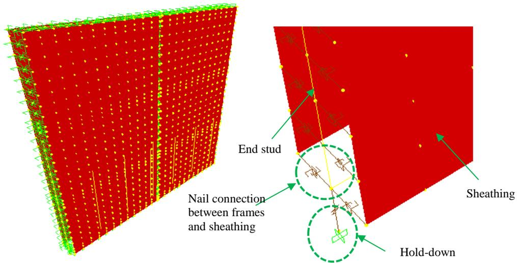
Figure 3. Wood frame shear wall model configuration in SAP2000
