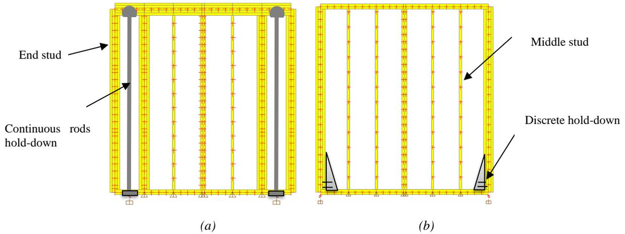
Figure 2. Wood frame shear walls configuration (a): continuous steel rods, (b): discrete hold-downs according to [1], [4]
