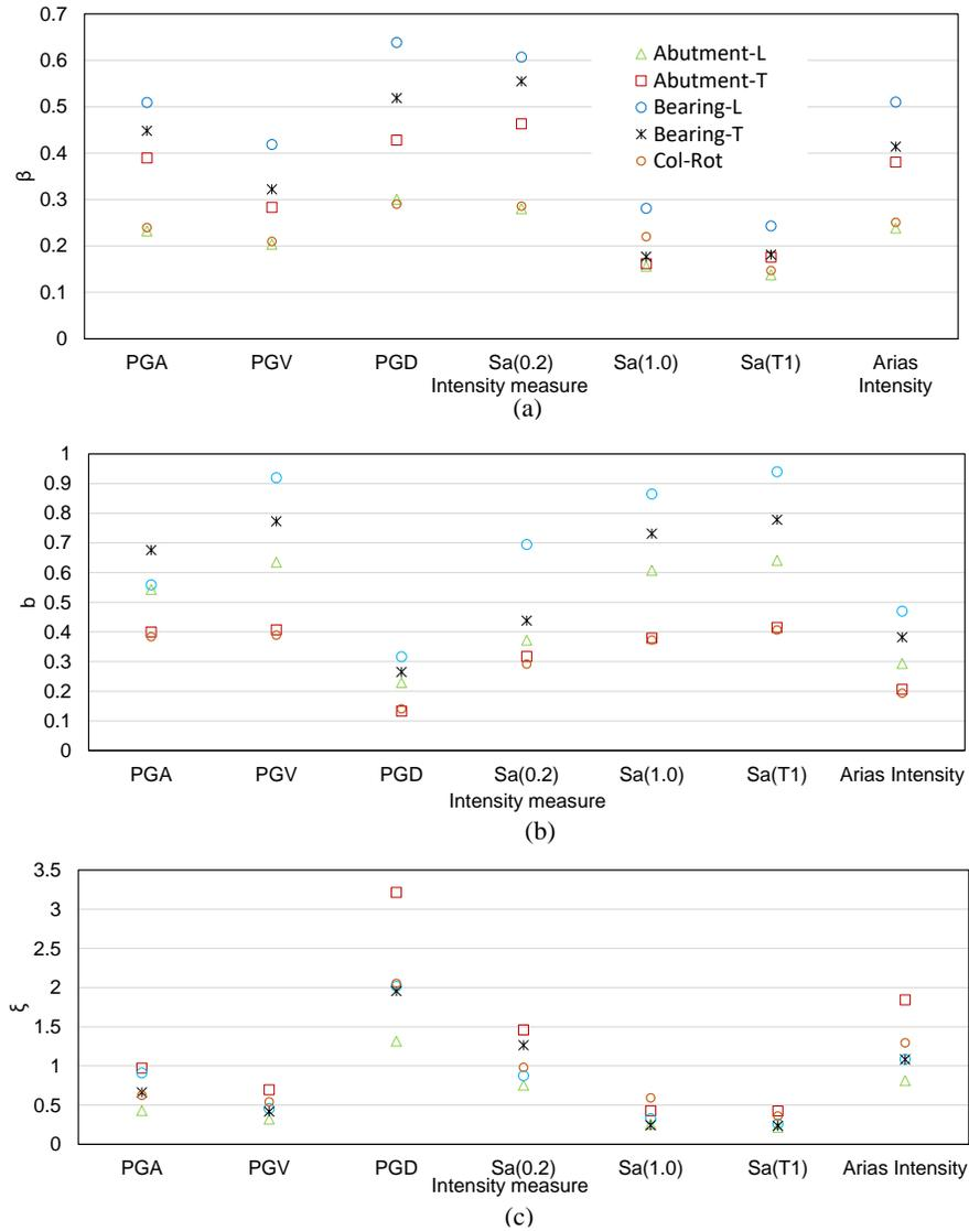
Figure 5. The efficiency, practicality, and proficiency evaluation for considered IMs and demands under LD New Zealand earthquake
