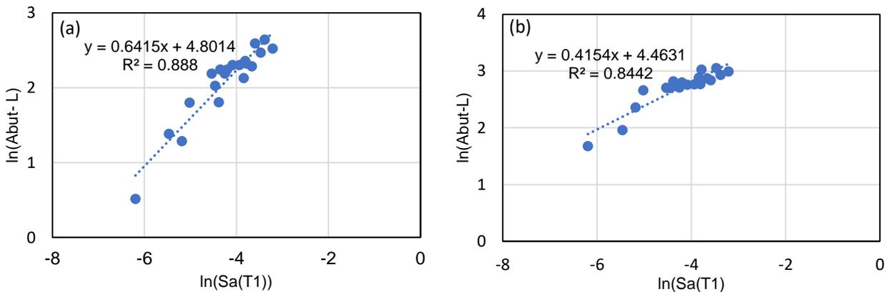
Figure 3. The plotted diagram and the fitted regression line for the abutment deformation and the intensity measure of  $S_a(T_1)$
