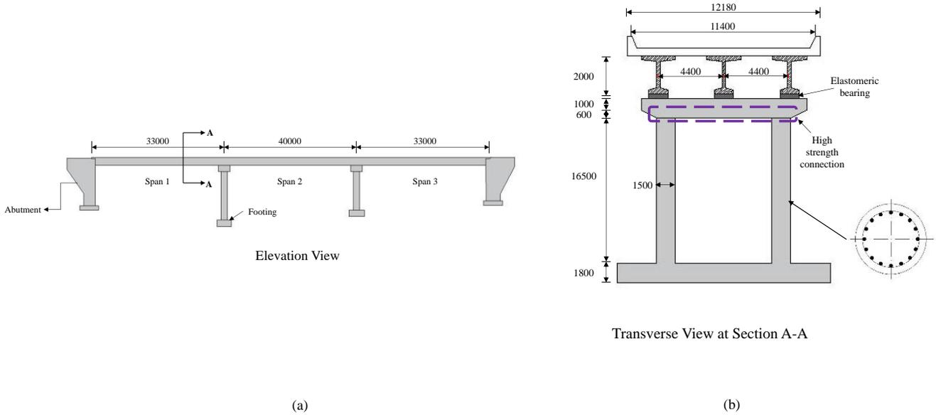
Figure 2. Dimensions of the bridge: (a) Elevation view, (b) Transverse view at section A-A.
