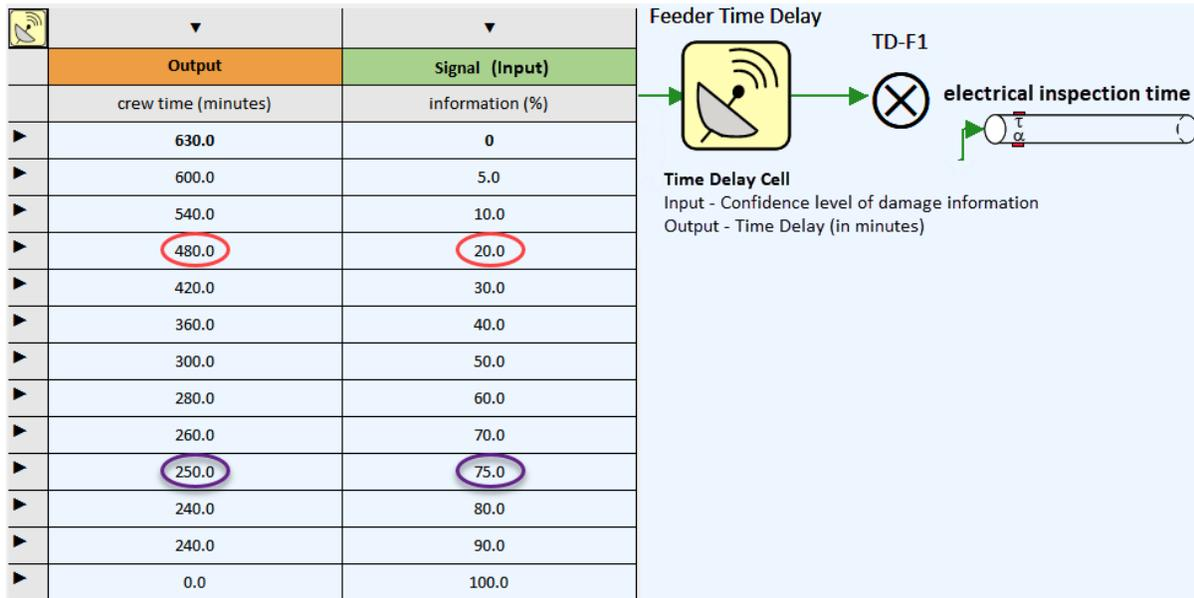
Figure 5. The HRT controlling the Channel's time delay for the electrical crew inspection time; the input is the confidence level of the damage information, and the output is the time delay of the crew (in minutes).
