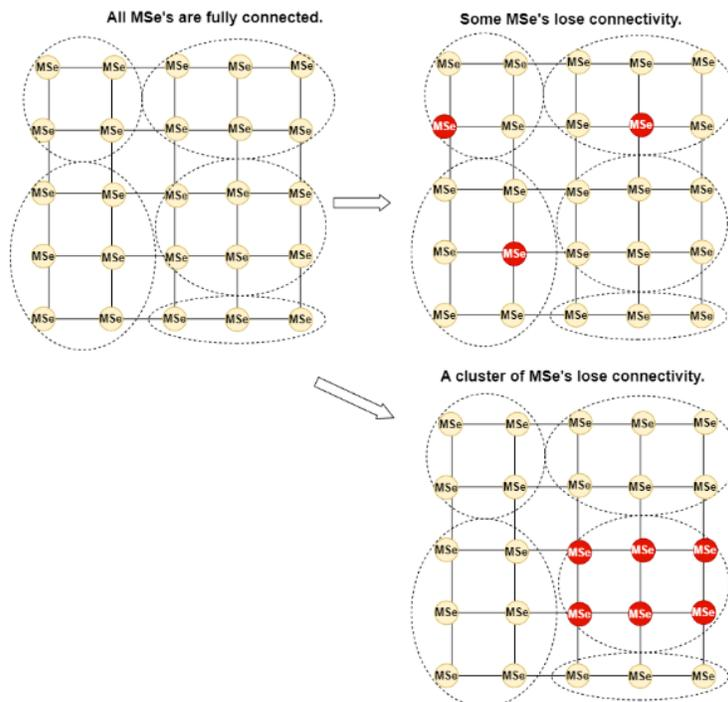
Figure 2. Failure of sensor stations: (a) Left – all sensors are working and capturing the waveform data (b) Top-Right – a few stations have lost connectivity, (c) Bottom-Right – a whole MEC has lost connectivity.
