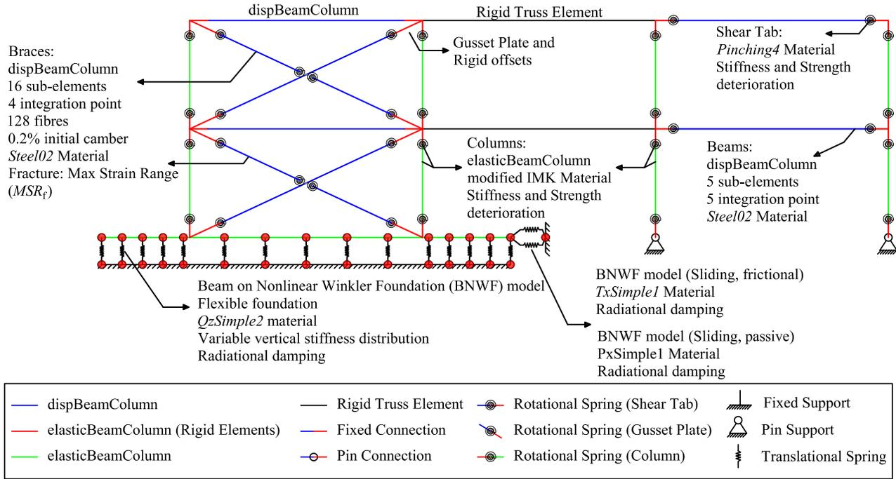
Figure 2 Analytical model of structure-foundation-soil system
