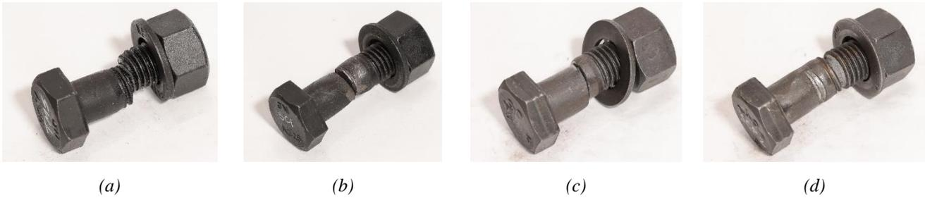
Figure 4. Bolt Test Damage: (a) A325 3/4" Threads Monotonic, (b) A325 3/4" Shank Cyclic, (c) A490 1" Shank Monotonic, (d) A490 1" Shank Cyclic Pretensioned
