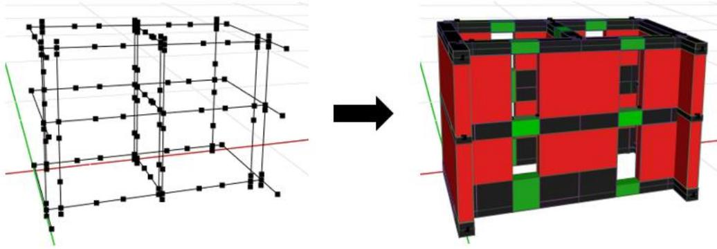
Fig. 3 : Discretization of the building into equivalent frames following the Augenti approach.
