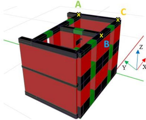
Fig. 4: 3D Model of SSF template. Points A, B and C are those used as control points in the pushover analysis.
