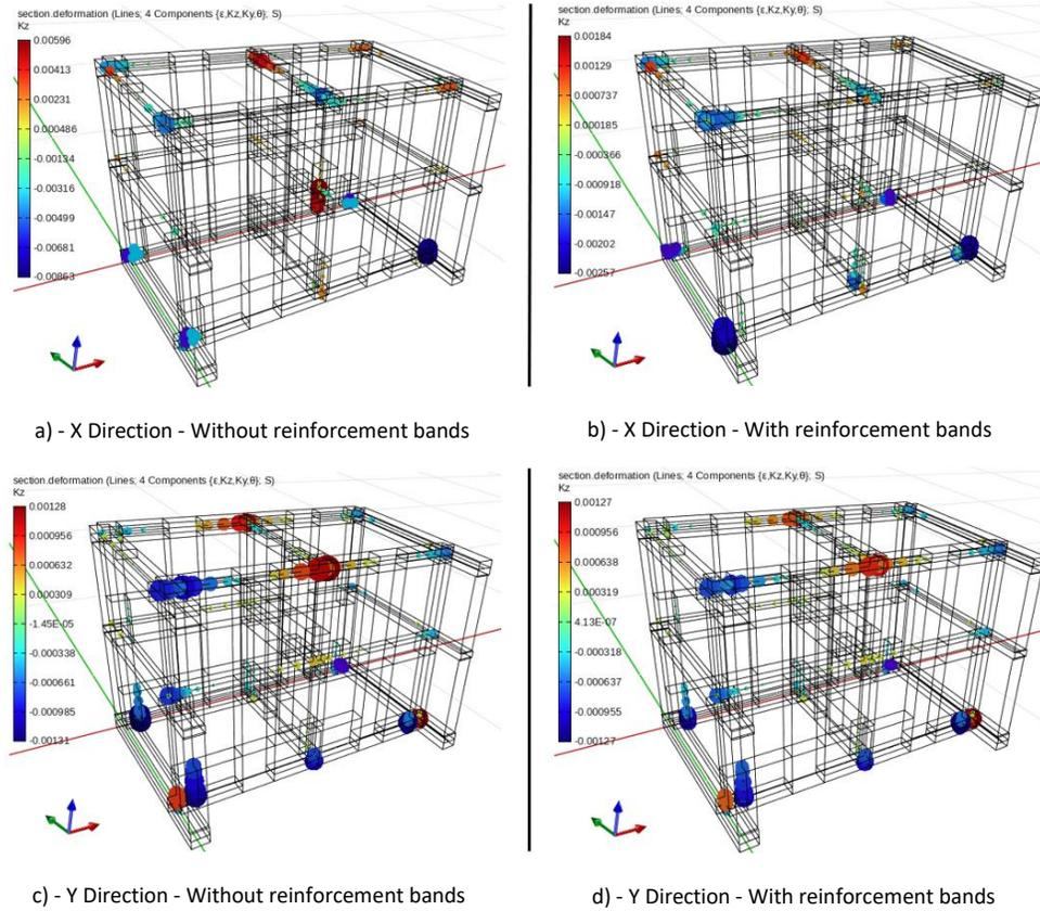
Fig. 6 : Sequence of plastic hinges formation according to the two configurations: (a) with and (b) without additional bands
