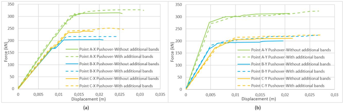
Fig. 5 : Pushover curve of the SSF template with RC bands in (a) X direction and (b) Y direction captures at three control points A, B, C
