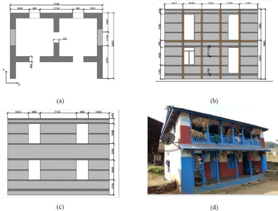
Fig. 1: Two-story Smart Shelter template: (a) plan view of the ground floor; (b) front elevation; (c) back elevation; (d) photograph of a completed building in Nepal.
