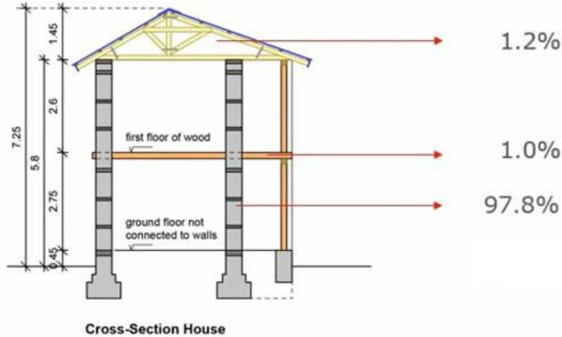
Fig. 2 : Seismic weight concentration in the typical SSF building. (adapted from [8])
