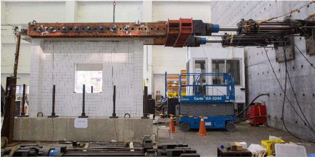
Figure 5. Test setup and the physical sub-structure of the retrofitted RC frame hybrid model
