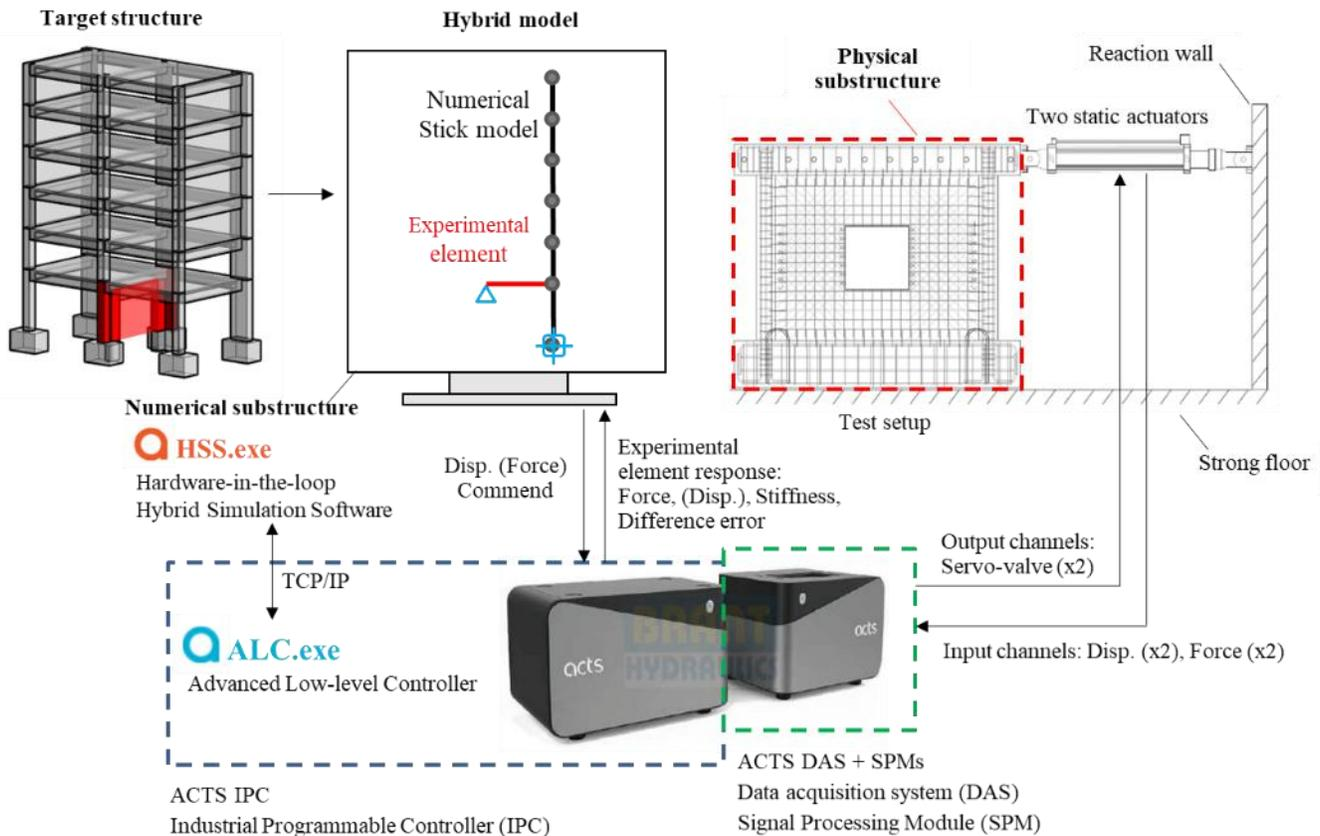
Figure 4. Hybrid simulation architecture diagram
