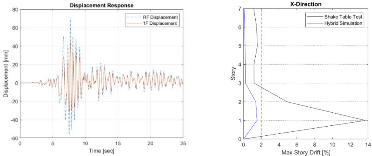
Figure 8. Testing results of the retrofitted prototype RC building after CHY063 800 gal, (a) first-storey and roof displacement history, and (b) storey drift ratio of the prototype building with and without retrofitting.
