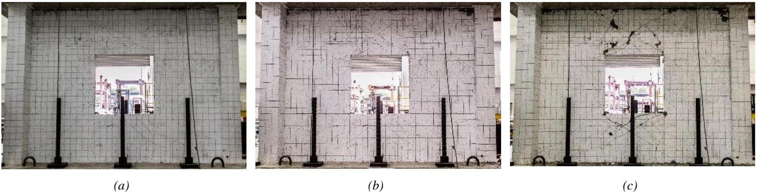
Figure 7. Crack pattern of Front view of the RC wall with opening after (a) CHY063 400 gal, (b) CHY063 600 gal, and (c) CHY063 800 gal.
