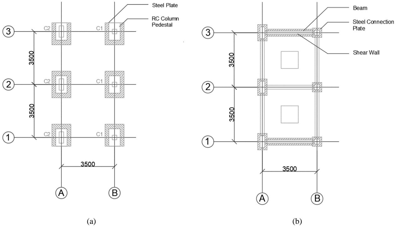
Figure A1. Plan view of the 7-storey prototype building (a) the first two stories, and (b) the third to seventh stories. [unit is in mm]
