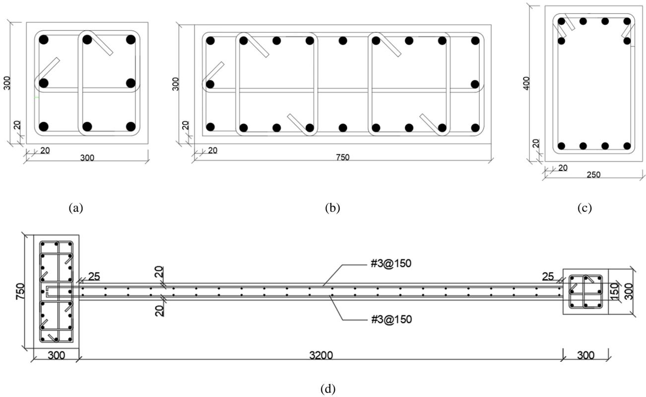
Figure A2. Cross-sectional dimensions of (a) square columns, (b) rectangular columns, (c) beams, and (d) infilled shear walls. [unit is in mm]
