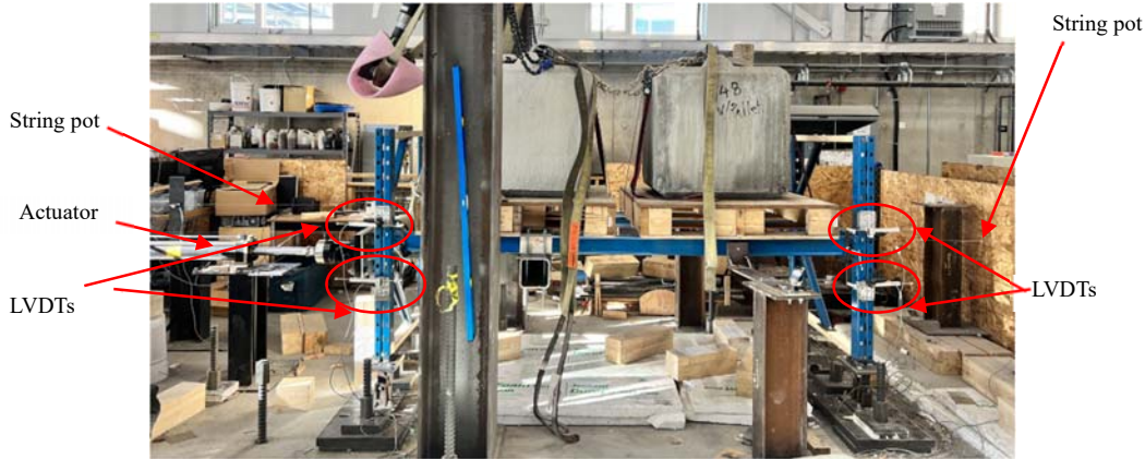
Figure 3: Instrumentation of the portal frame test.
