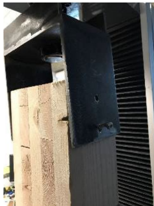
Figure 15. Screws pull-out during the tests
