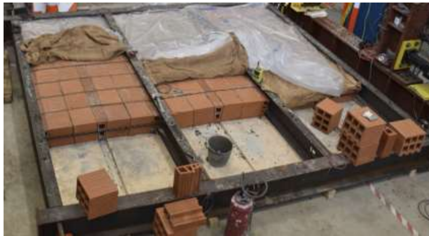
Figure 2: A sample of a multi-panel terra cotta floor constructed in the NRC's structural lab
