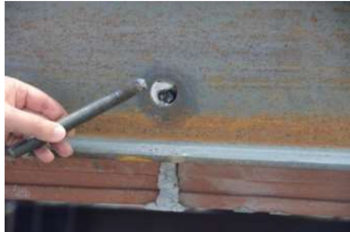
Figure 8. Tie-rod failure in multi-panel test MB3
