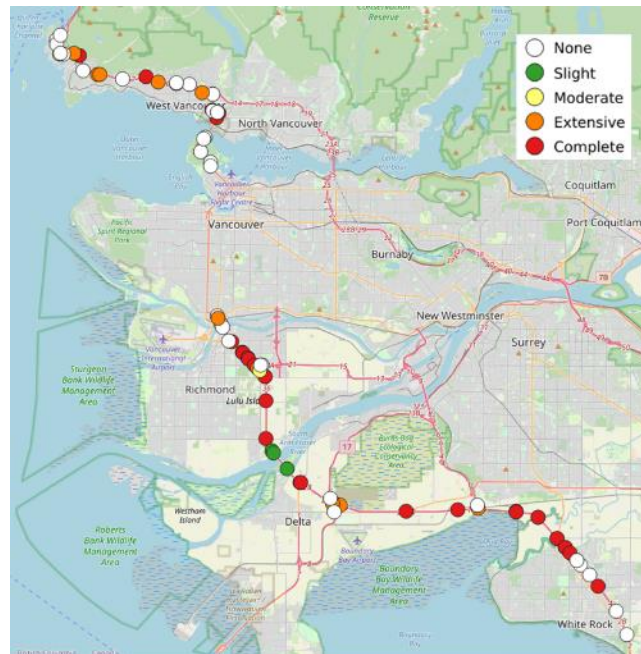
Figure 6. Median Damage to Bridges for the Subduction Scenario.
