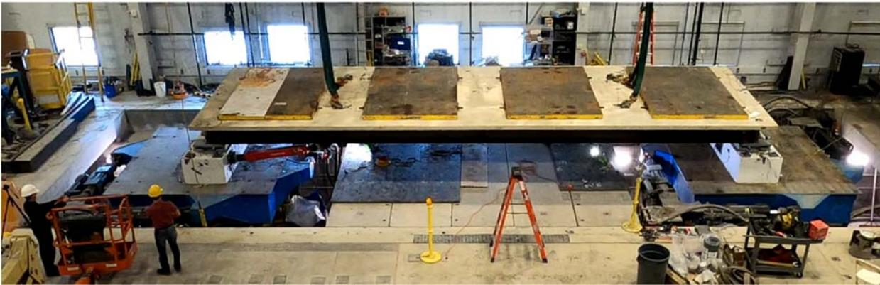
Figure 5: Specimen set up on top of the two shake tables
