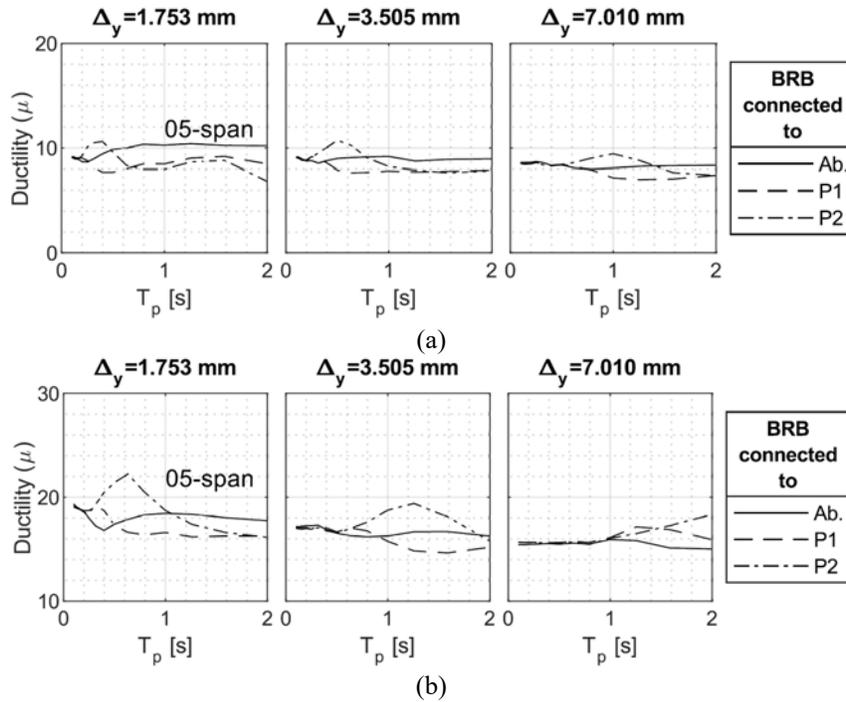
Figure 2: 90th percentile of BRB ductility demands in bridges with target ductilities equal to: a) 5, b) 10
