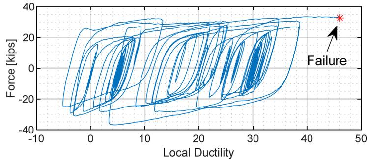
Figure 8: Preliminary hysteretic loop of a BRB from a few ground motions before its failure (note: this is “truncated” data; for clarity, the hysteretic curves corresponding to all the ground motions tests applied to this BRB are not all included in this figure)
