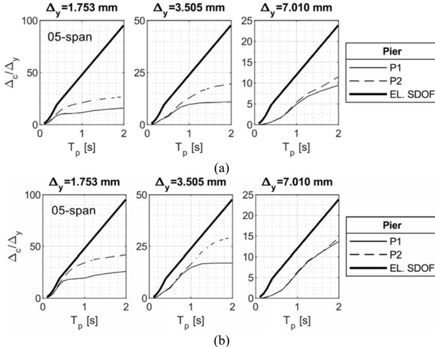
Figure 3: Displacement demand of piers in bridges with target ductility equal to 10: a) mean, b) 90th percentile
