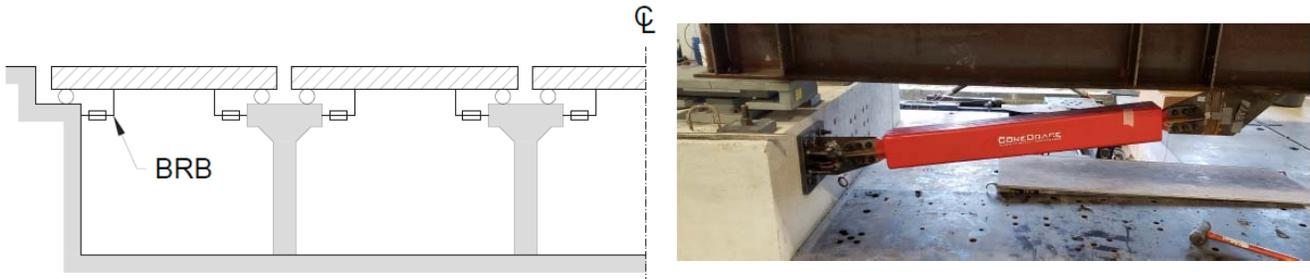
Figure 1: Bridge: a) Scheme, b) Example implementation of a BRB in the longitudinal direction, connecting bridge span to abutment or pier cap
