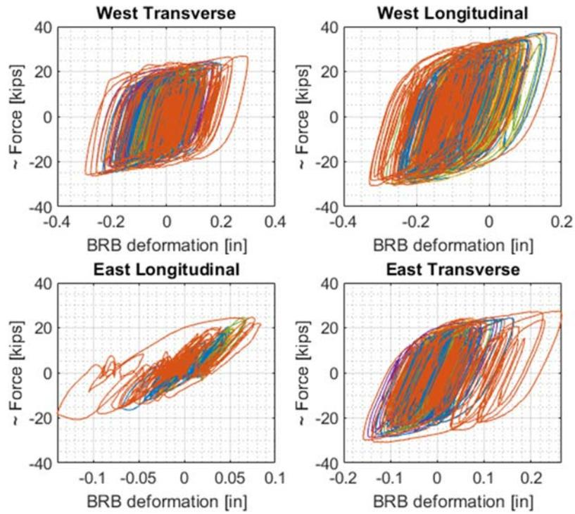
Figure 7: BRB hysteretic loops for the steps 1 – 61 for Configuration I
