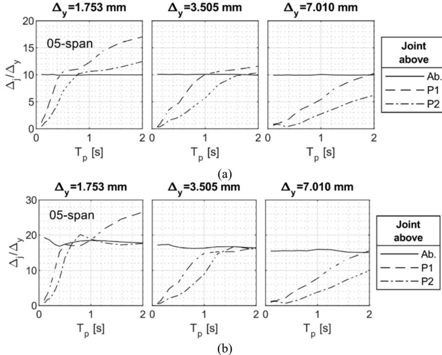
Figure 4: Expansion Joints demands in bridges with target ductility equal to 10: a) mean, b) 90th percentile
