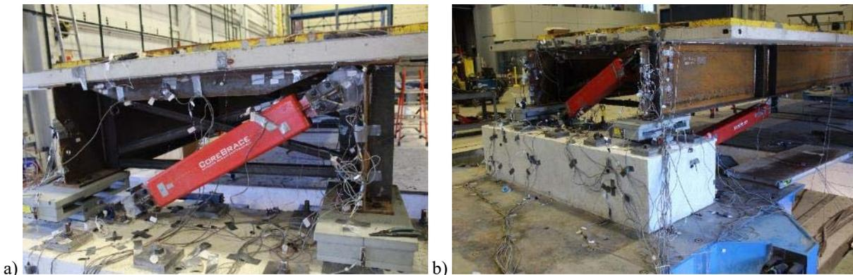
Figure 6: Specimen with BRBs and instrumentation for Configuration I: a) transverse BRB in the west end, b) longitudinal BRB
