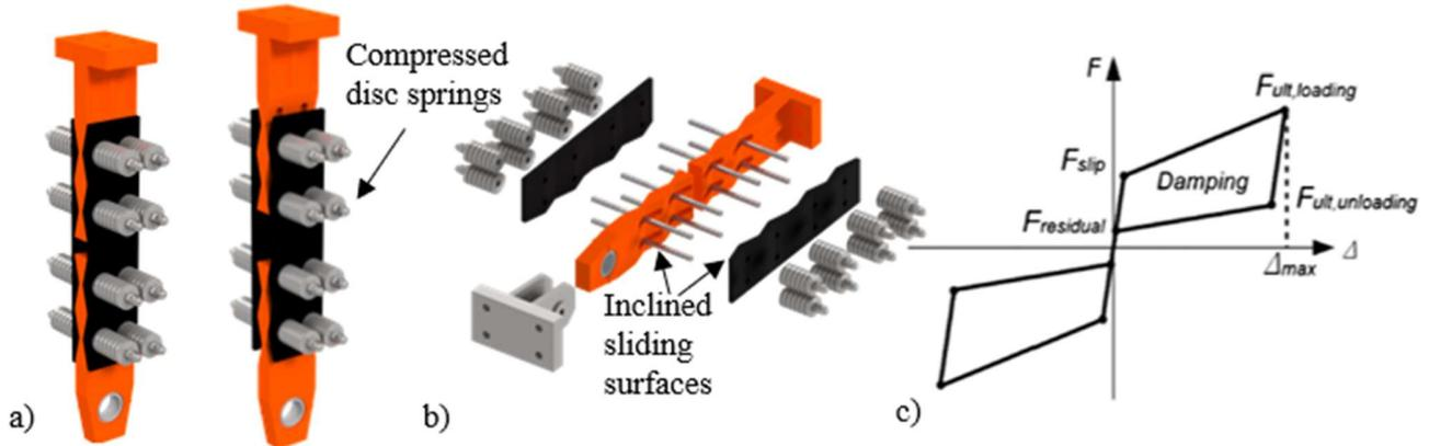
Figure 2 a)RSFJ Hold-down at rest and Extension b) Component Details c) Hold-down hysteresis
