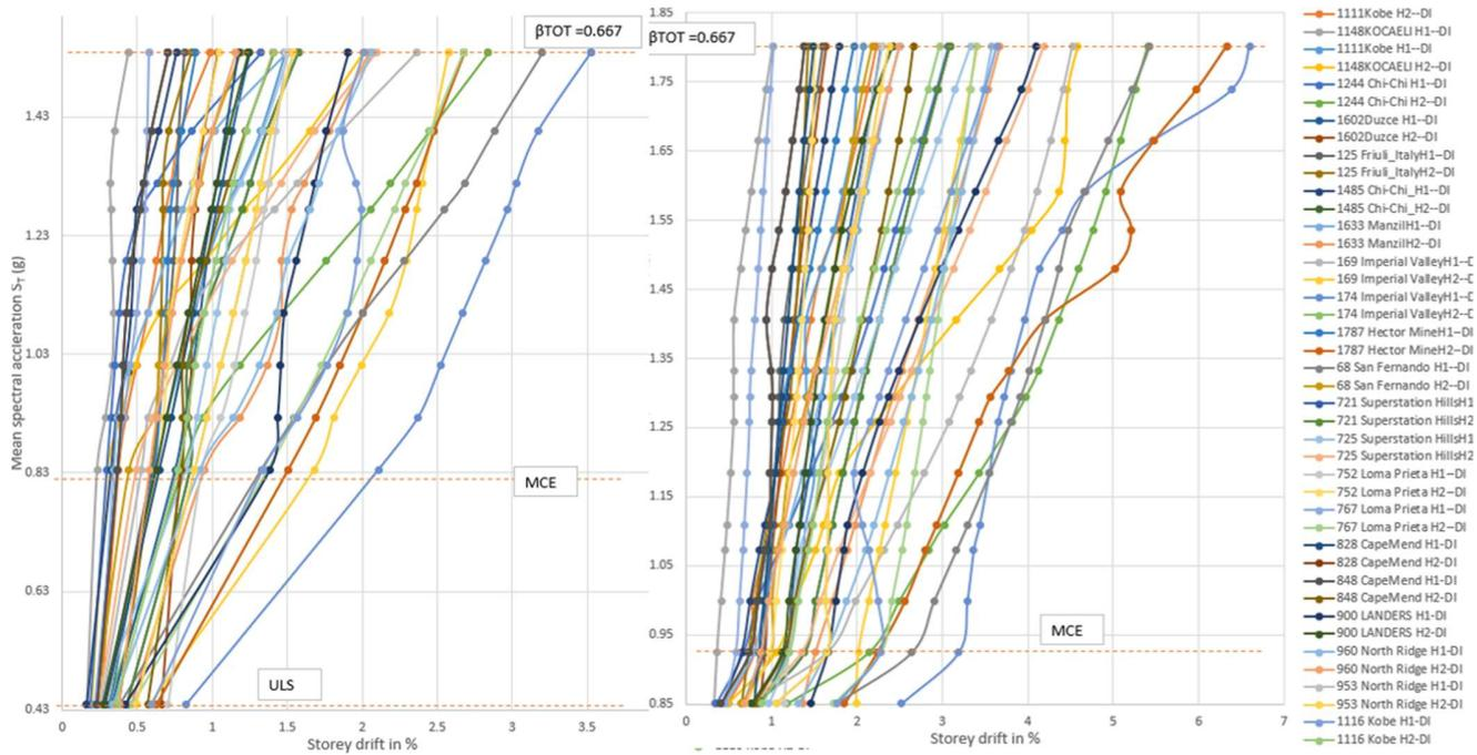
Figure 5 Collapse evaluation – IDA for 10-storey coupled wall-wall LLRS (left) and 10-storey coupled wall-column LLRS (right).
