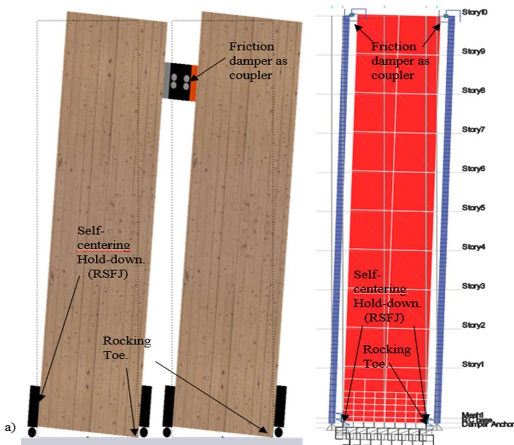
Figure 1 a) Coupled-wall with wall. b) Coupled wall with boundary columns
