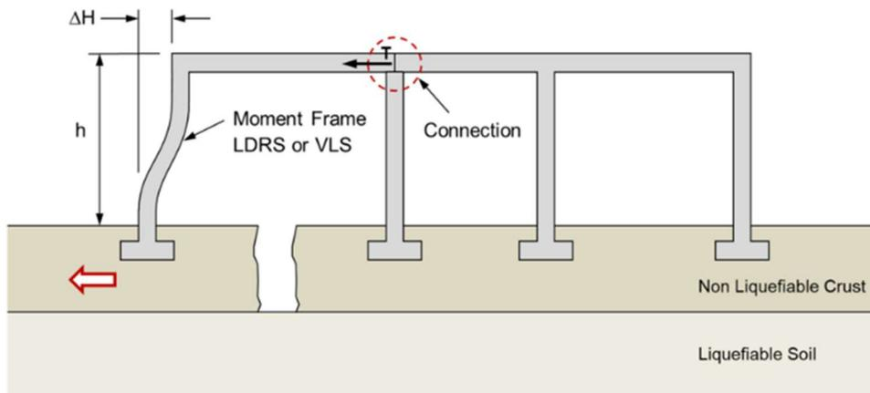
Figure 7. Lateral Soil Spreading Effects for Condition 1: Moment Frame LDRS and VLS
