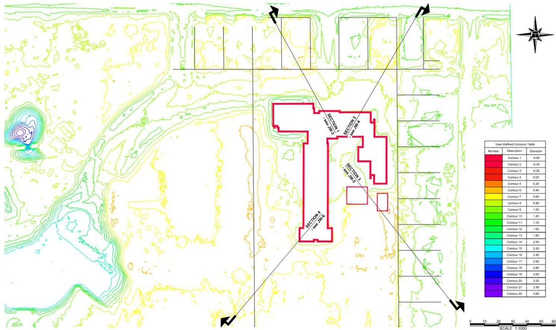
Figure 1. Example of Processed LiDAR Survey Showing Local Topography Surrounding School on Inland Floodplain Site
