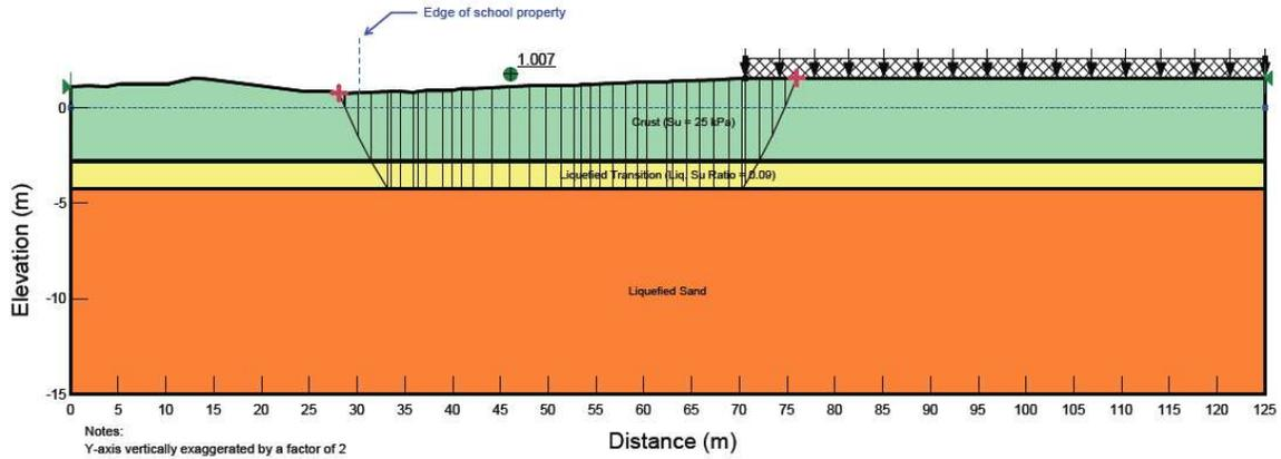
Figure 3. Example Limit Equilibrium Analysis to Determine Yield Acceleration of the Governing Slip Surface
