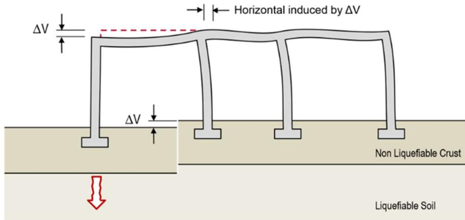
Figure 8. Differential Vertical Settlement Effects for Condition 1: Moment Frame LDRS and VLS
