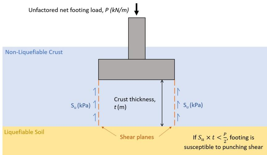
Figure 4. Illustration of Punching Shear Assessment
