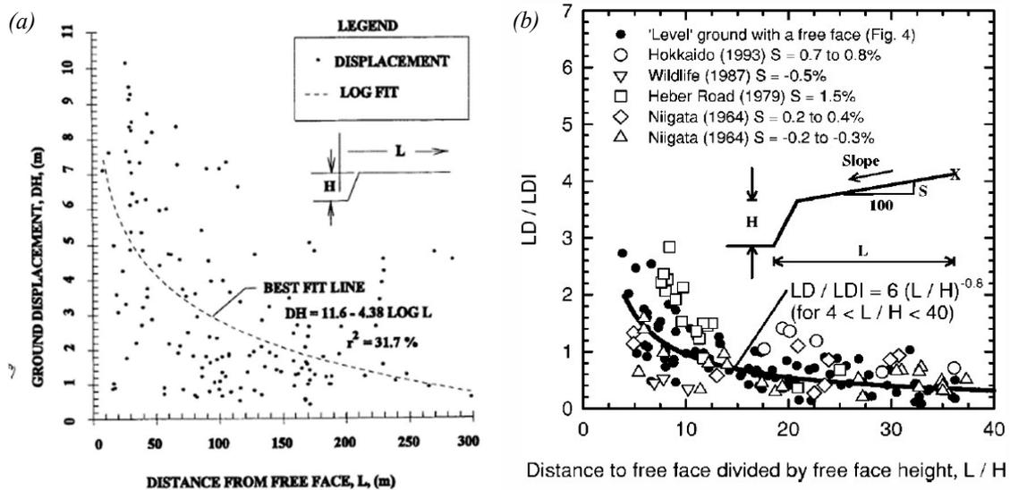
Figure 2. Observed Lateral Ground Displacement as a Function of Set Back from Free Face Feature from (a) Bartlett and Youd (1995) and (b) Zhang et al. (2004)
