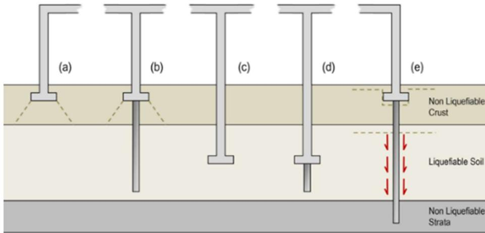
Figure 5. Foundations Located in Crust or in Liquefiable Soil
