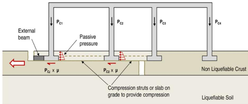
Figure 10. Possible Friction and Soil Pressure Loads
