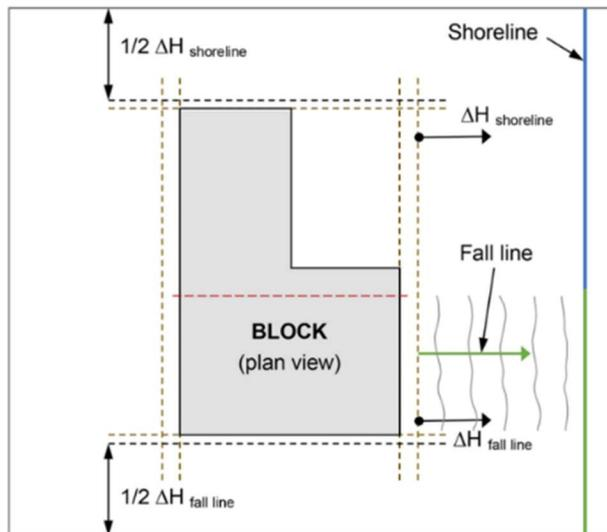
Figure 6. Lateral Soil Spreading Effects for Shoreline and Fall Line
