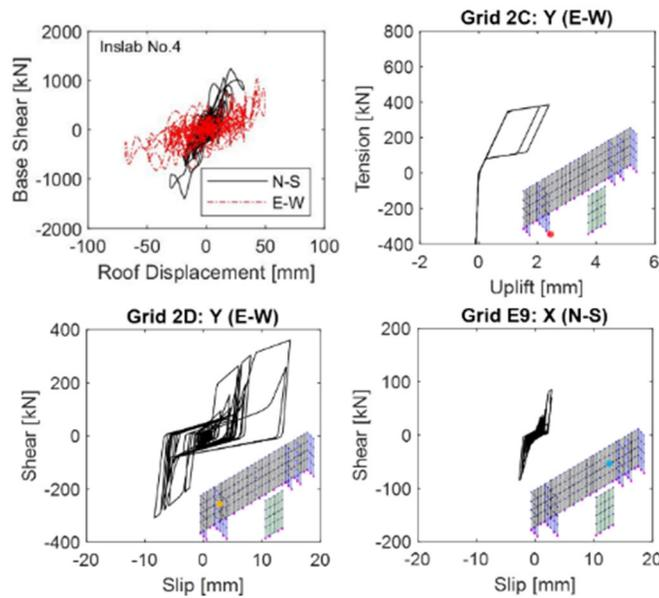
Figure 8: Nonlinear hysteresis curves of the building and connections during subduction inslab motion.
