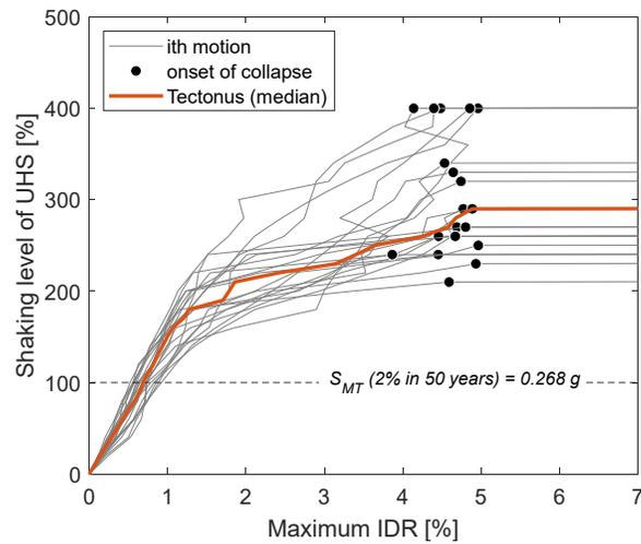
Figure 9: IDA curves of building model.
