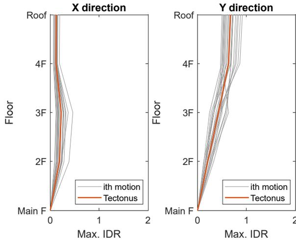
Figure 7: Maximum IDR at design level.
