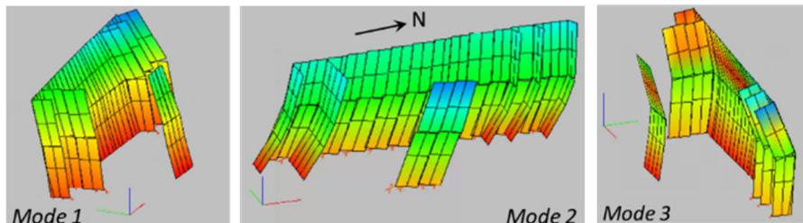
Figure 6. Mode shapes of the building model.
