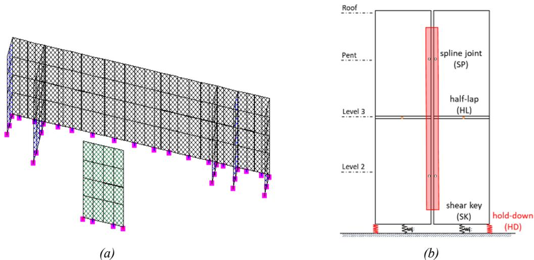
Figure 3. OpenSees building model: (a) 3D model, (b) 2D balloon-framed CLT shear wall model.
