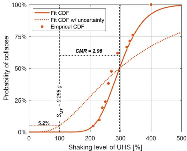
Figure 10: Collapse fragility curve with uncertainty.
