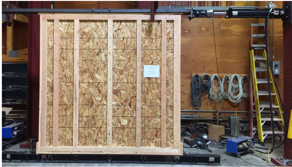
Figure 8. Test setup with a Midply specimen ready for testing.
