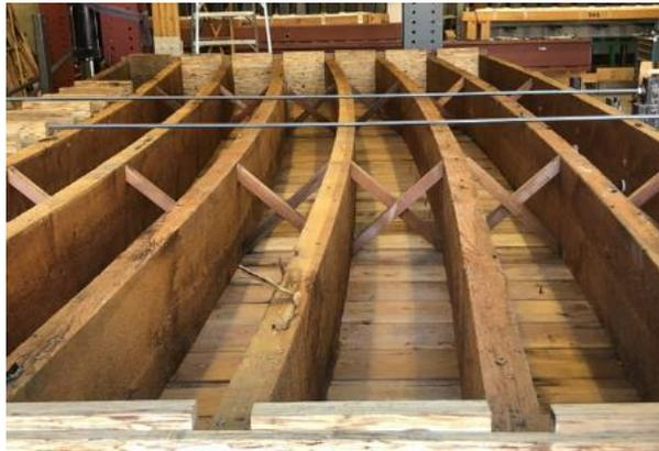
Figure 12. Deformation of the roof deck joists.
