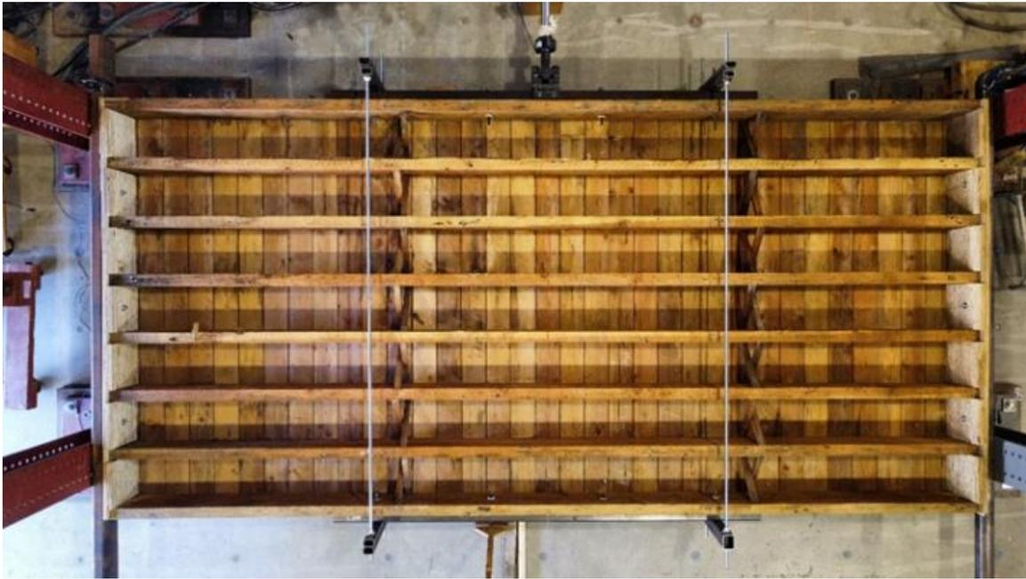
Figure 8. Test setup for the roof deck specimen reversed cyclic testing.
