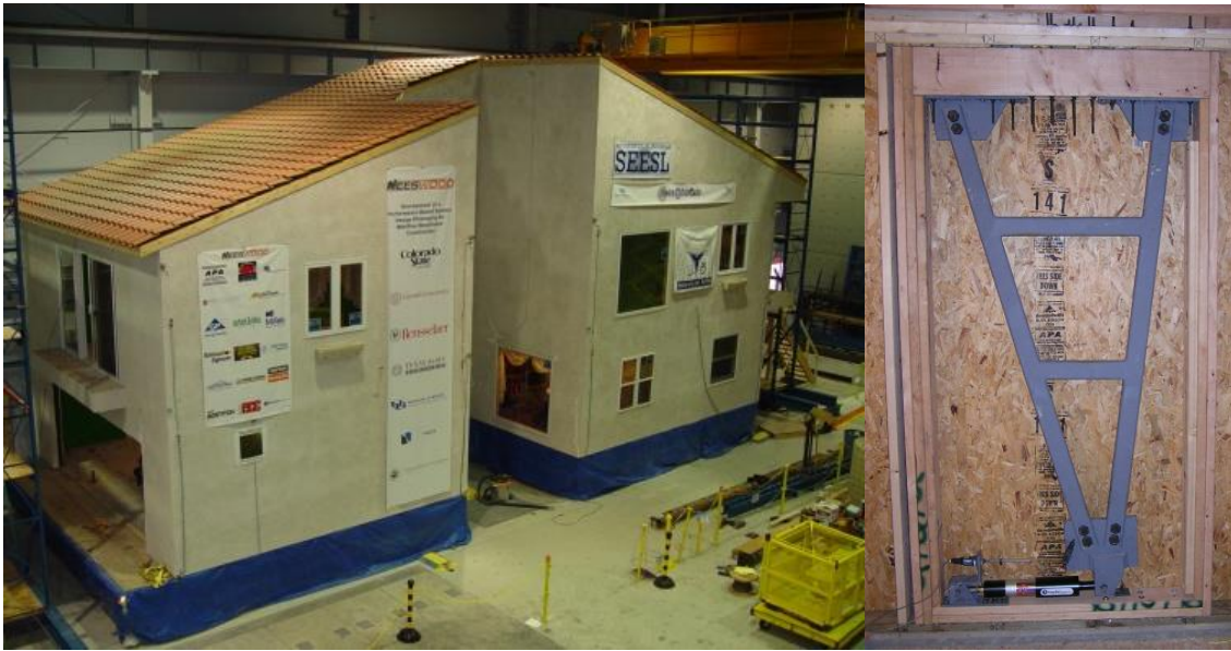
Figure 3. NEESWood building model and modular damper wall [6]
