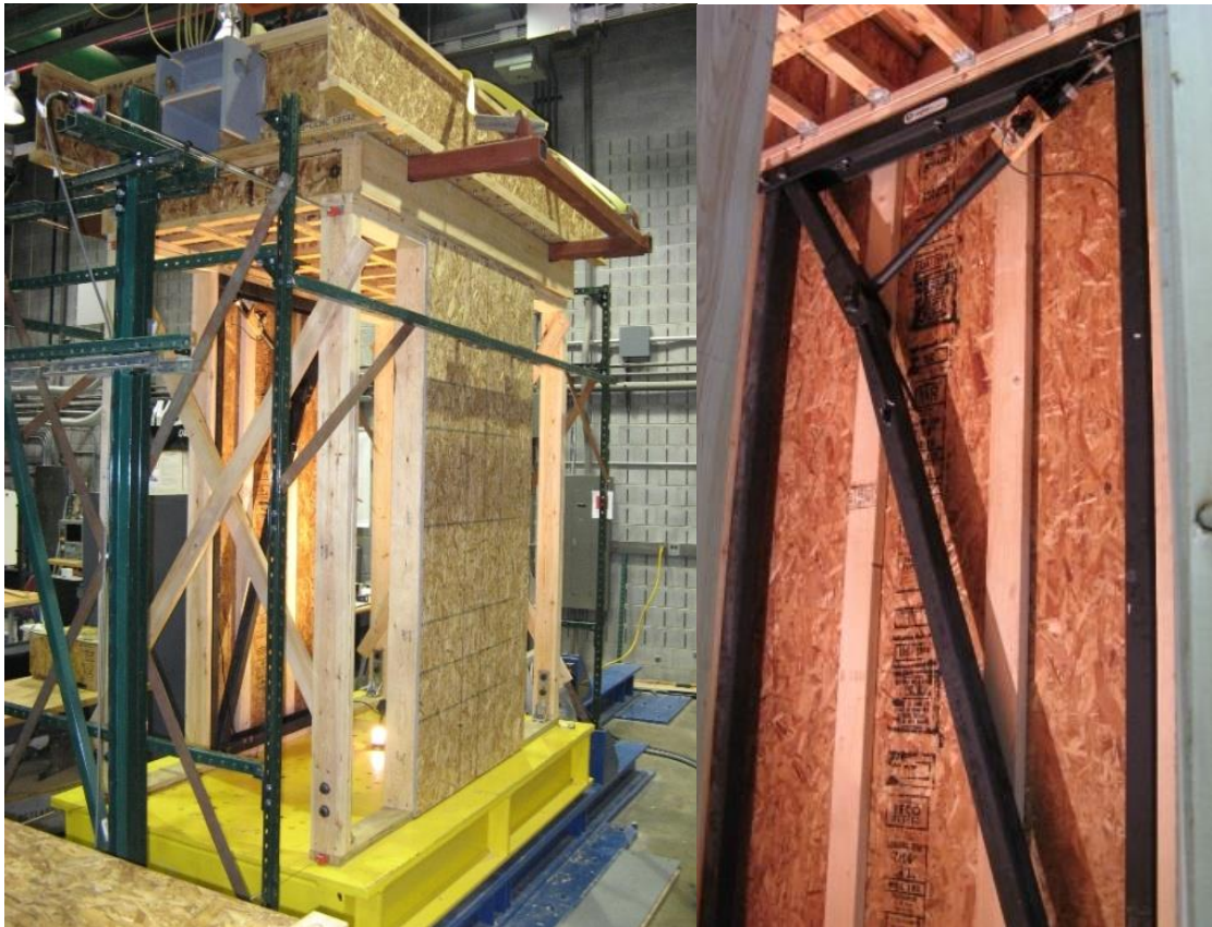
Figure 4. NEESWood model retrofitted wall and toggle-braced damper [6]
