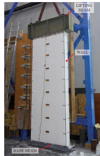
Fig. 20 Typical Wall Specimen Prior to Testing (Penner 2014)
