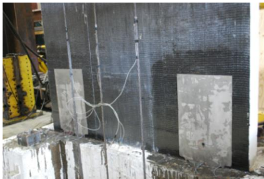
d) Anchors on the Wall Surface
