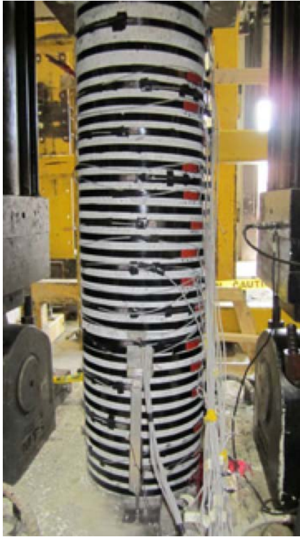
(a) Typical retrofitted column
