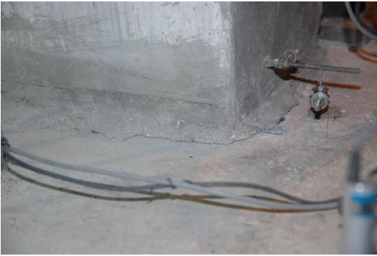
a) Observed Cracks at different drift ratio levels
