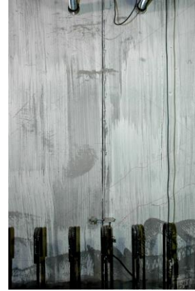
b) View of interface at drift ratio of 0.20%
