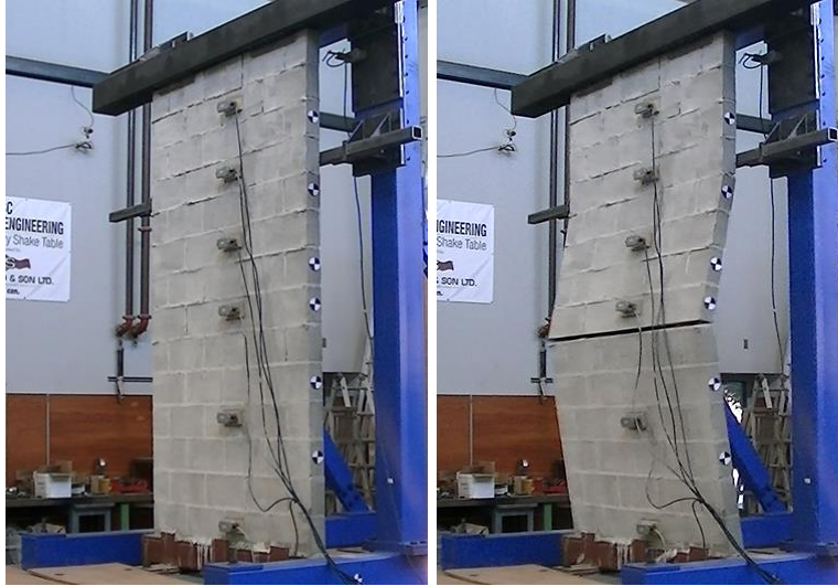
Fig. 2 - Failure Locations of Horizontal Restraint Wall
