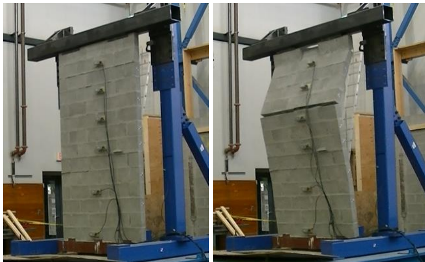
Fig. 1 – Failure Location for Bare Wall
