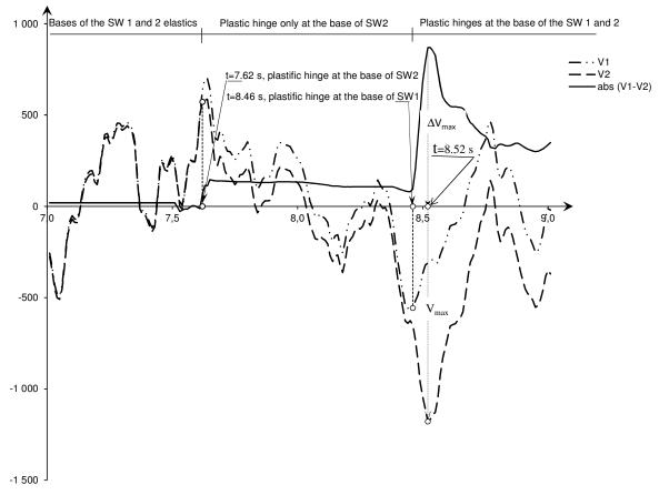
Fig. 4 – Typical evolution of the distribution of shear demand between SW1 and SW2 (kN)
