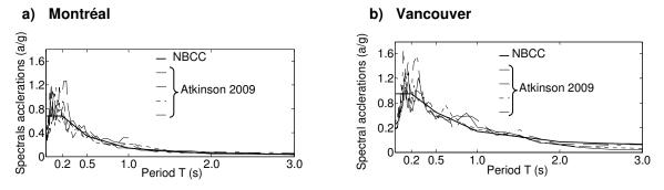
Fig. 2 – Seismic signals (Atkinson 2009) calibrated compatible to acceleration spectrum
