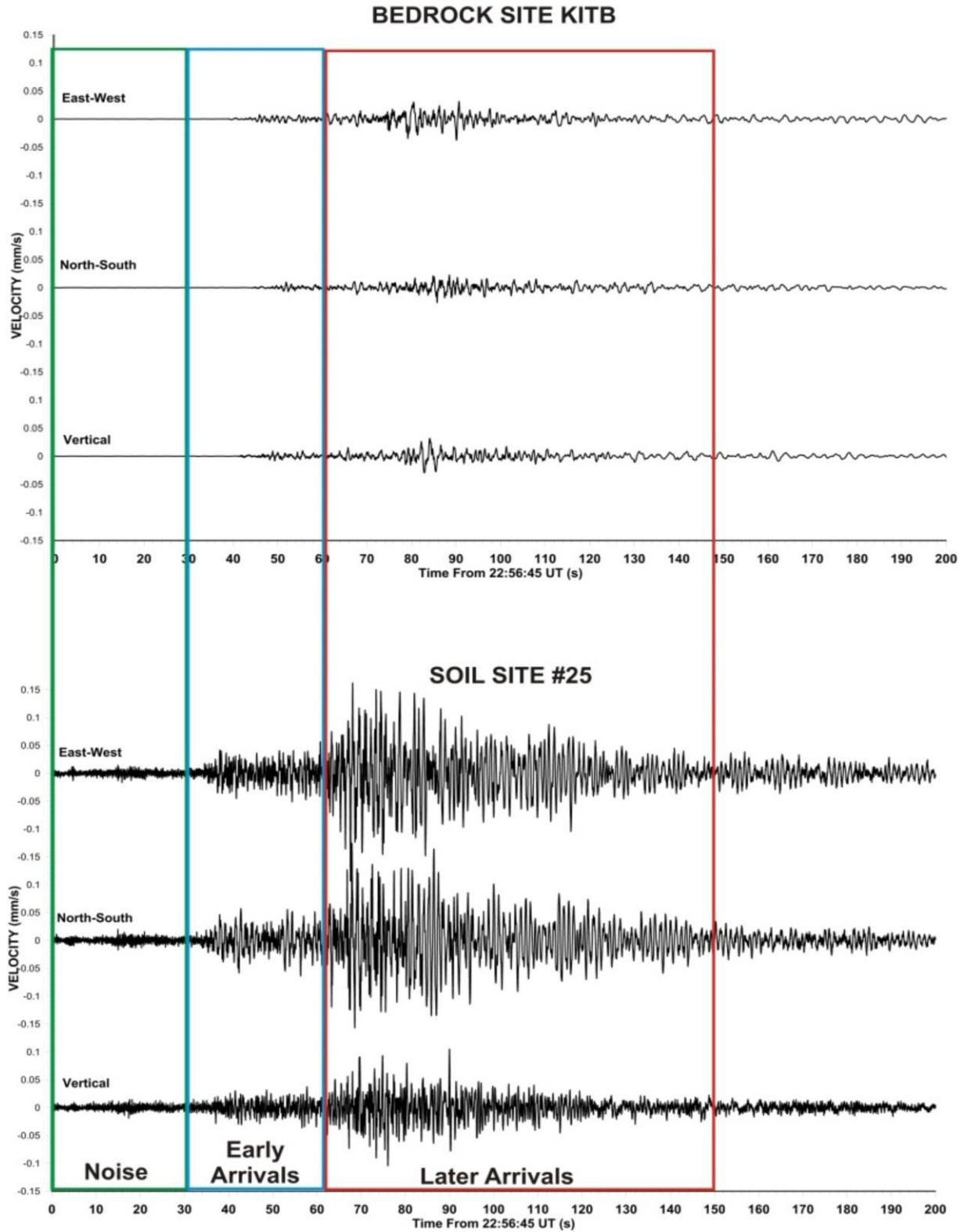
Fig. 4 - Three-component ground velocity seismograph records (pass band filtered 0.3 – 60 Hz) for the bedrock site KITB and the Tromino soil site KIT-25. All traces shown at the same gain levels.
