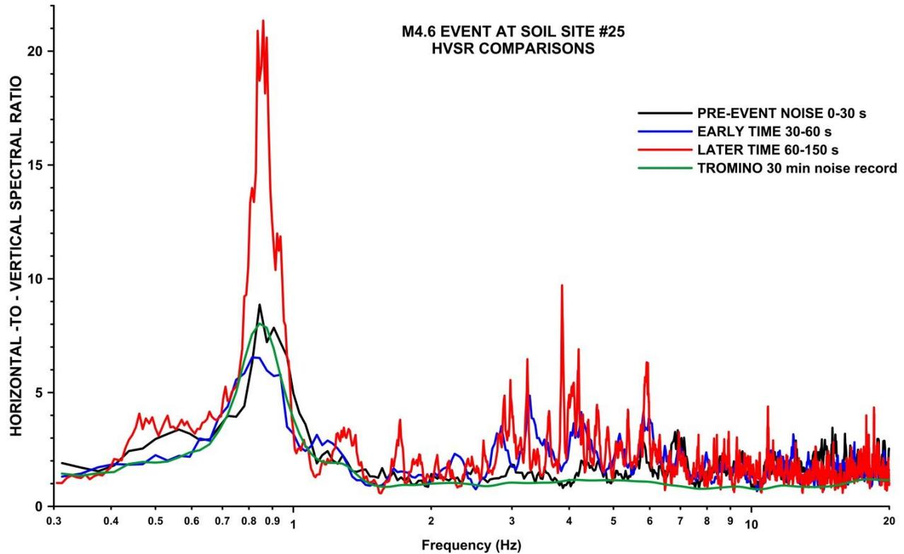
**Fig. 5 - HVSr for the  $M_w$  4.6 earthquake event time windows (as shown in Fig. 4) recorded at soil site KIT-25, compared to the 30 minute ambient noise recording.**
