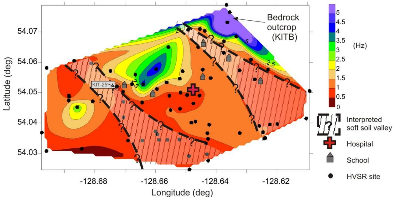
**Fig. 3 – Map showing fundamental site frequencies within the town of Kitimat. Heavy dashed lines indicate the inferred boundaries of soft soil valleys. Areas in red (frequencies <1 Hz) are located over thick soil deposits. Site KIT-25 indicates where the portable seismograph recorded the  $M_w$  4.6 earthquake.**
