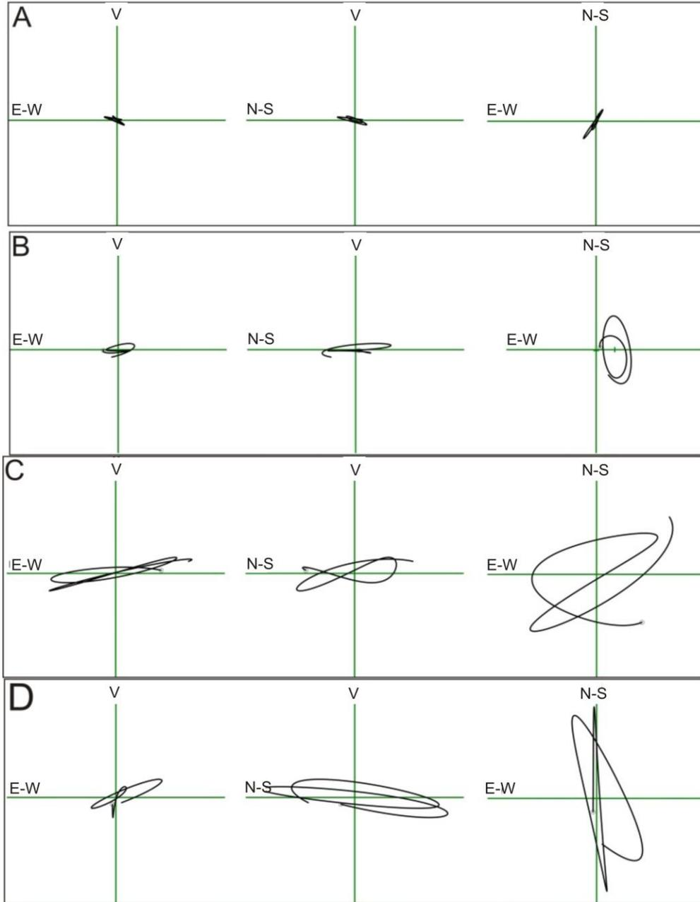
**Fig. 6 - Particle motion plots of (A) First P- wave arrival, (B) shear wave, (C)-surface wave motion - azimuth 45°, (D) surface wave motion - azimuth 340°.**
