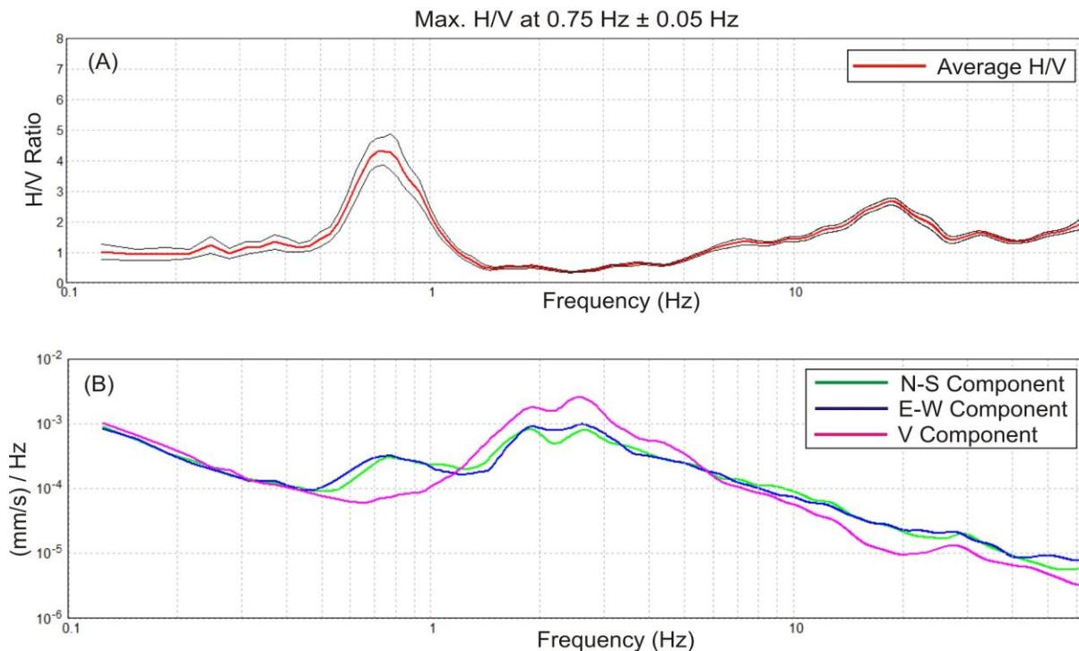
**Fig. 2 – (A) Sample H/V spectral ratio for site KIT2-27 (B) North-south, east-west, and vertical average spectra for the windows used in the HVSr interpretation. Note that there is amplification on the vertical component, but it lags behind the horizontal components on the frequency axis which creates the dominant peak in panel A.**
