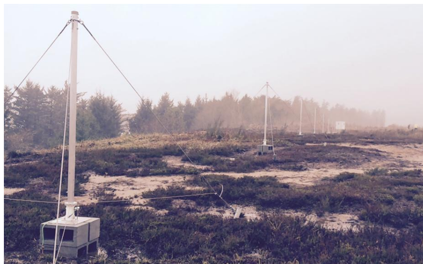
Fig. 2 – WERA system installed in Long Beach Airport, Tofino, British Columbia
