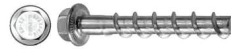
USE: (2) HILTI KWIK HUS-EZ \phi = 1/2" CARBON STEEL SCREW ANCHOR MIN. EMBEDMENT: 1-1/2" [KH-EZ 1/2" x 2-1/2"]
