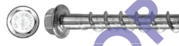
USE: (2) HILTI KWIK HUS-EZ \phi = 1/2" CARBON STEEL SCREW ANCHOR MIN. EMBEDMENT: 1-1/2" [KH-EZ 1/2" x 2-1/2"]
