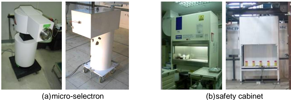
Fig. 3 – Experimental specimen for the selected medical equipment for shaking table tests
