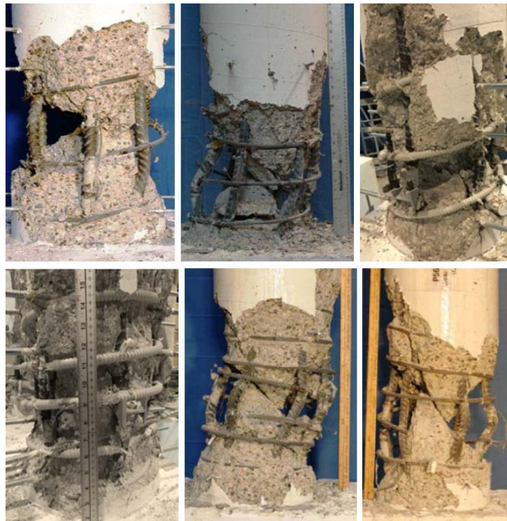
Fig. 7 – Columns after testing (in clockwise direction, starting from top left): P27-NF-1, P27-NF-2, P28-LS-12-160, P56-NF-11, P56-NF-12, and P55-LS-12-90
