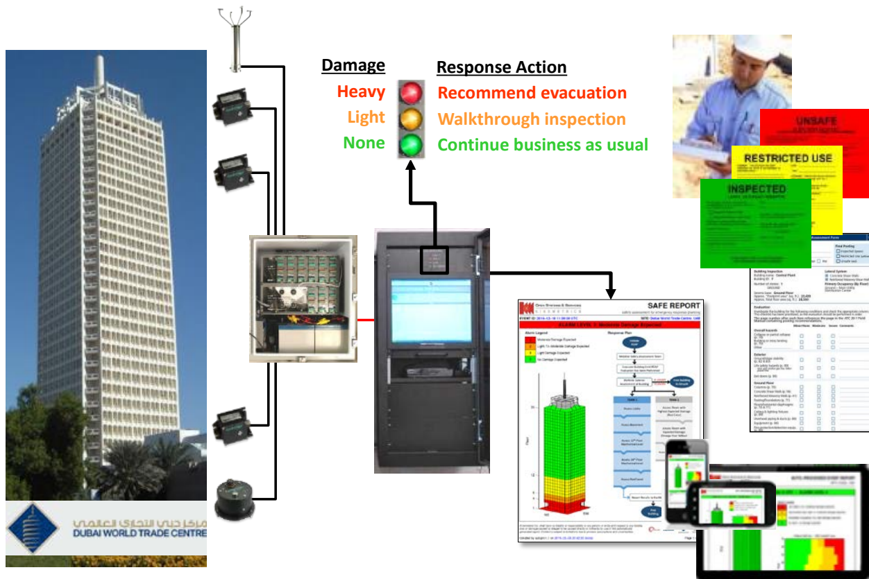
Fig. 3 – OASIS structural health monitoring system.
