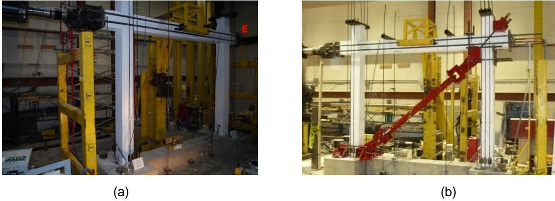
Figure 5: Loading setup prior to testing: a) control frame; and b) retrofitted frame
