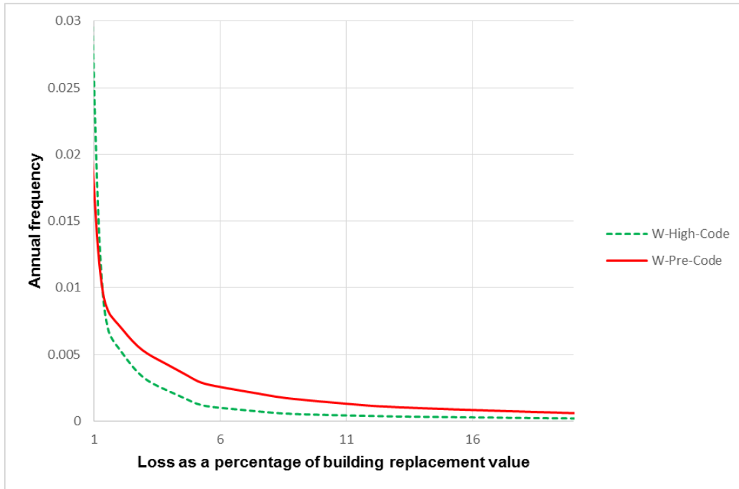
Fig. 2 – Annual frequencies of losses for 2 wooden buildings in the City of Vancouver.
